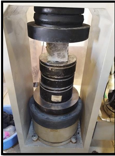
Figure III. 7: Essai de compression de Béton
