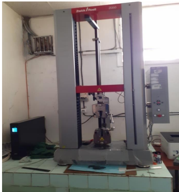
Figure II.2. Machine de traction ZWICK ROELLZ050
