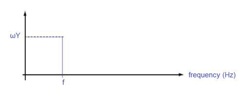
figure (2-4): Frequency representation of the vibration speed(12).
