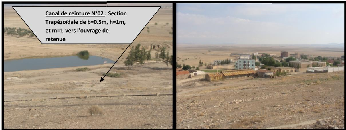
**Figure IV N° 09 Canal de Ceinture N°02**
