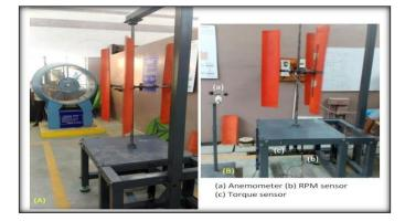
Figure 2.14: (a) Experimental setup (b) Close view of the proposed VAWT in test rig. [22]
