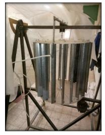
Figure 3.2: Fabricated model of quart-circular rotor montage H (twenty bladed).
