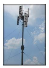
Figure 2.6: Prototype of the proposed Senegal VAWT.[18]
