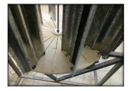
Figure 3.23: Twenty blades perpendicular to each other two by two.
