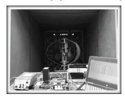
Figure 2.16: Performance investigation of hybrid VAWT within wind tunnel.[23]
