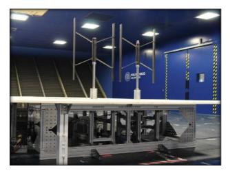
Figure 2.10: The two turbines were placed in their respective frames in the assembly. A floating floor was mounted on top of the boxes. [20]
