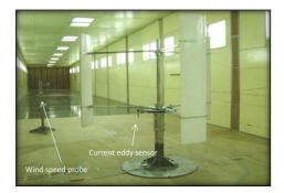
Figure 2.12: Wind turbine model installed in the wind tunnel.[21]
