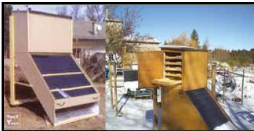
Figure (I-11): Séchoirs solaires indirects [7].
