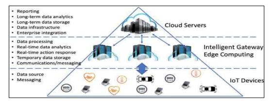
FIGURE 1.4. The basic edge computing architecture. [18]
