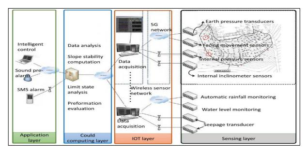
FIGURE 2.12. The hierarchical structure of early-alarm system for soil slope. [40]
