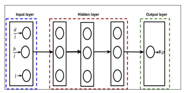
FIGURE 3.11. Schema of multi-layer perceptron regressor (MLPRegressor).
