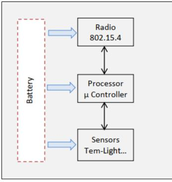
Figure 29: Block diagram of TelosB sensor
