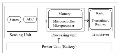
Figure 3: Sensor node architecture [3].
