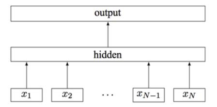
Figure 2.12: Model architecture of Fastext for sentence with n-gram features (Herwanto et al. 2019).
