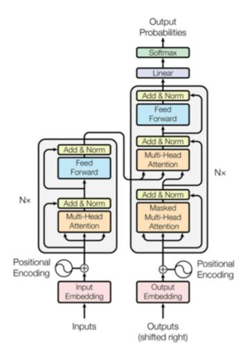
Figure 2.15: Transformer model architecture (Vaswani et al. 2018).
