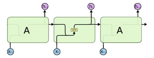
Figure 1.5: The repeating module in a standard RNN contains a single layer (F. Liu et al. 2019).
