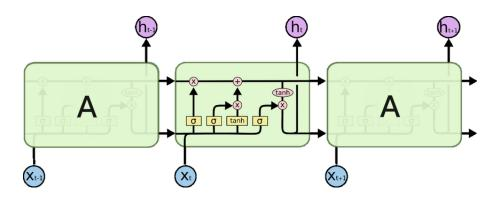
Figure 1.6: The repeating module in an LSTM contains four interacting layers (F. Liu et al. 2019).
