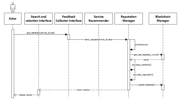
FIGURE 4.5: User give feedback sequence diagram
