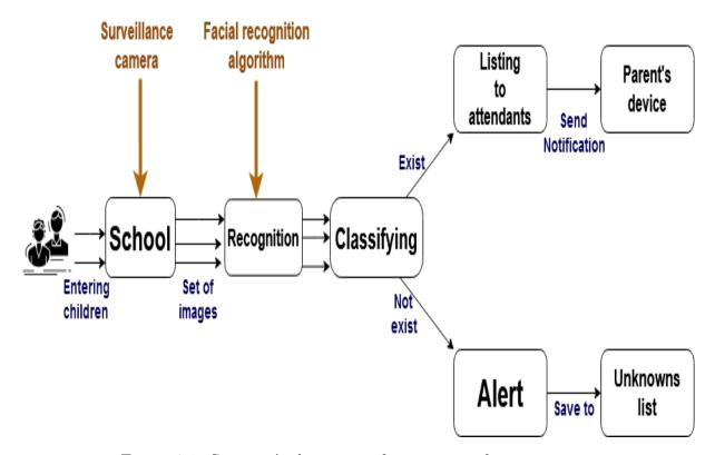
Figure 2.1: System Architecture of our proposed system.
