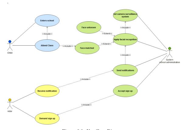
Figure 2.9: Use Case Diagram
