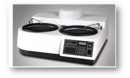
Figure (III.3): The polishing apparatus (polisher).
