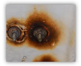
Figure (I.3): Schematic representation of crevice corrosion.
