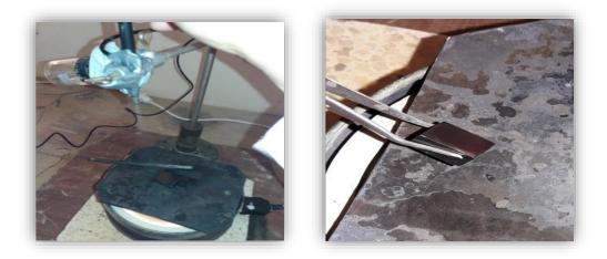
Figure (III.7): Thin layer on steel using the spray pyrolysis method.
