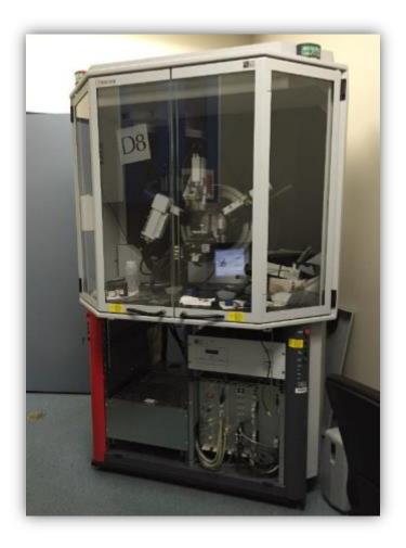
Figure (II.11): Photo of X-ray diffraction system.
