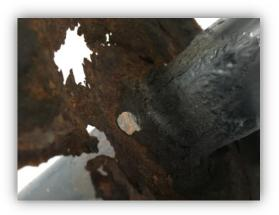
Figure (I.6): Schematic representation of selective leaching corrosion.
