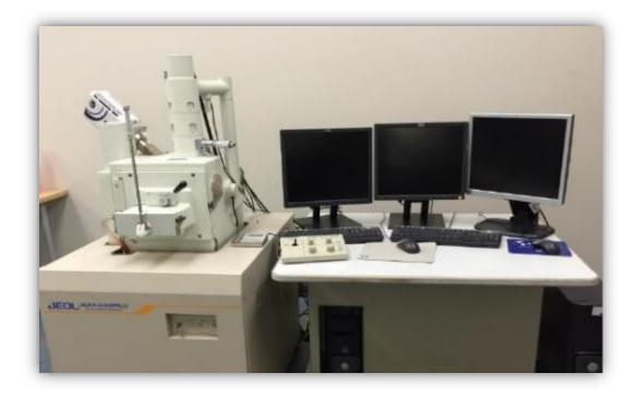
Figure (II.12): Photograph of the scanning electron microscope.
