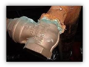
Figure (I.2): Schematic representation of galvanic corrosion.
