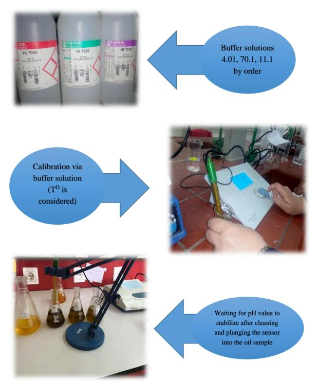
Figure 6: linseed oil pH measuring
