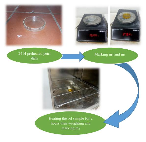
Figure 5: water rate measuring protocol
