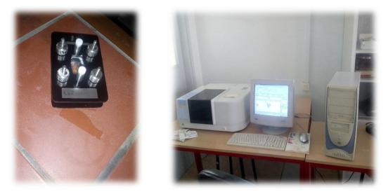
Finally you get to perform your FTIR analysis by launching the specified software (Shimadzu IR Solution) via PC and you get your spectrum.
