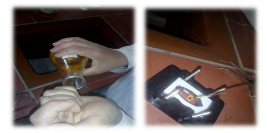
Close the support and introduce it to the spectrophotometer:
