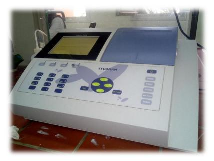
Figure 9: UviLine 9400 SECOMAM UV spectrophotometer
