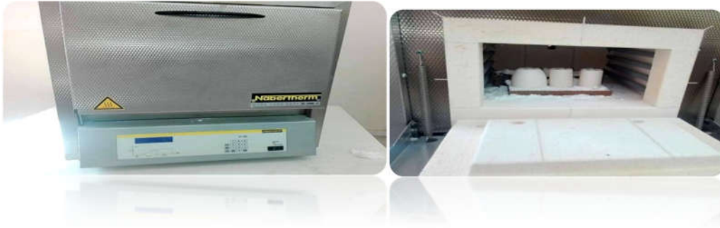
Figure II.6 : Outil de calcination.
