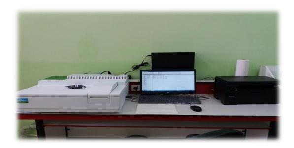
Figure 8: UV/VIS spectrophotometre
