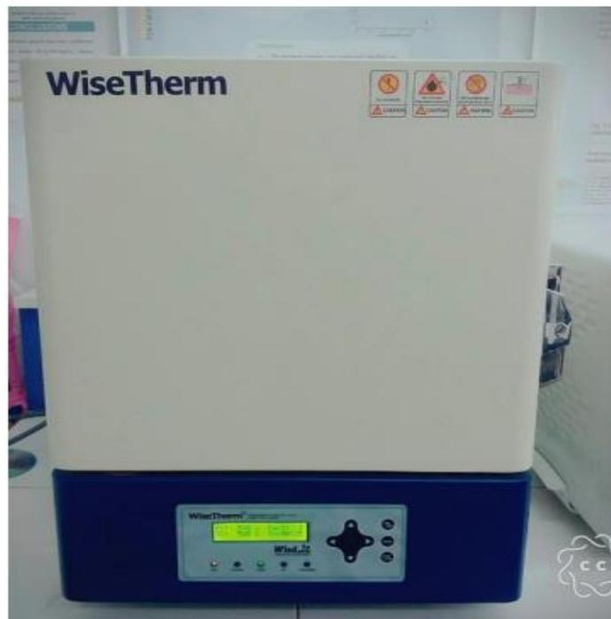
**Figure II.4:** Four de recuit. [42]
