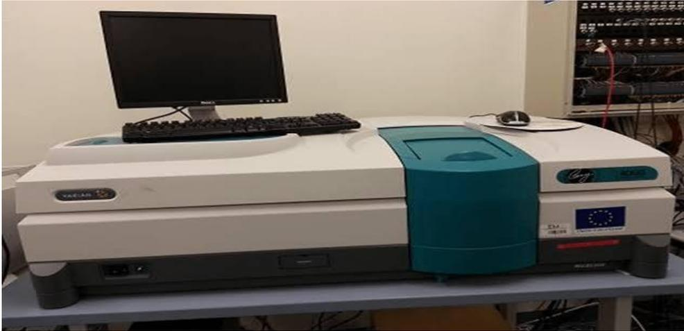
**Fig II.6 :** Ultraviolet-visible spectrophotometer [9]
