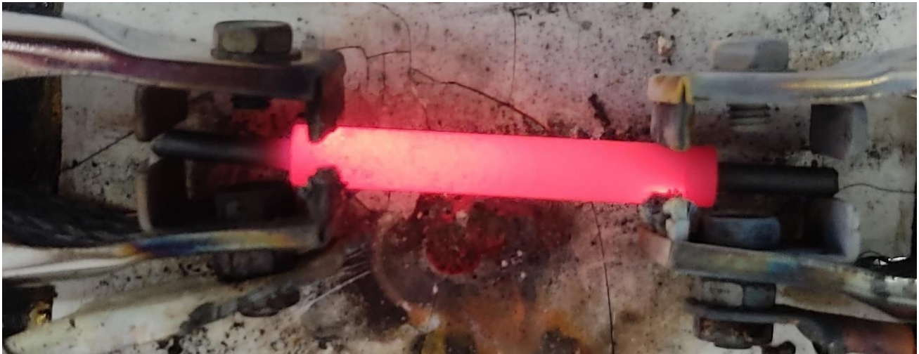
Figure 3.14. Iron powder pressed into a graphite die.
