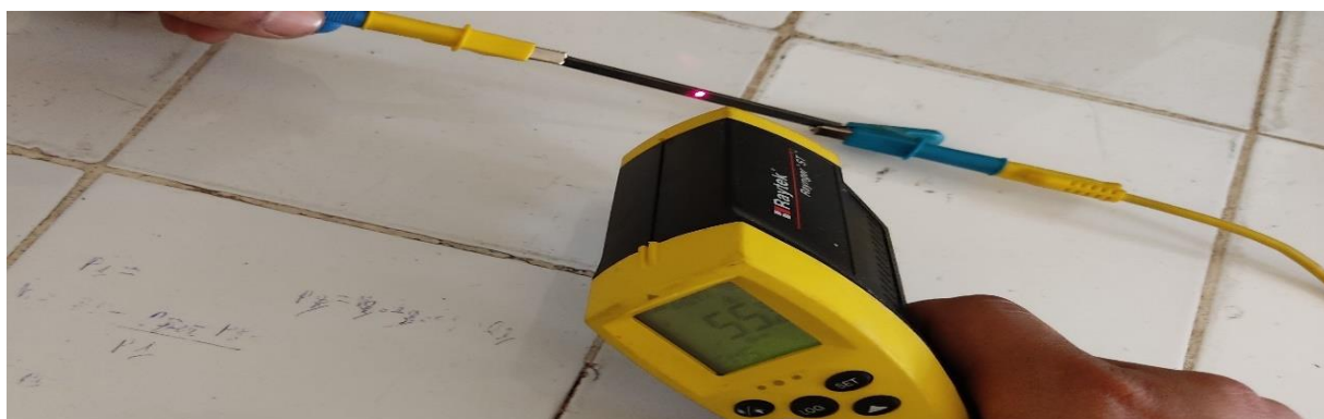
Figure 2.8. Graphite temperature measurement by Thermometer .
