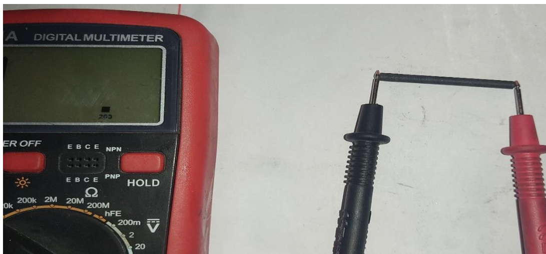
Figure 2.6. Measurement of the electrical conductivity of graphite by multimeter.
