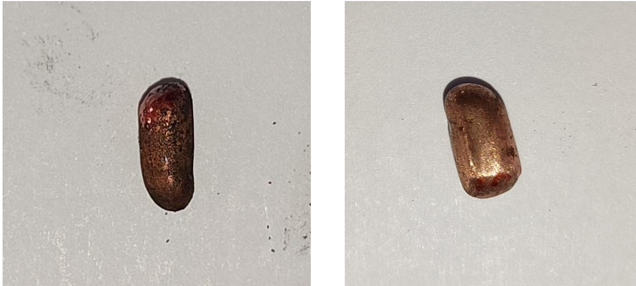
Figure 3.13. sintered copper powder (sample 2).
