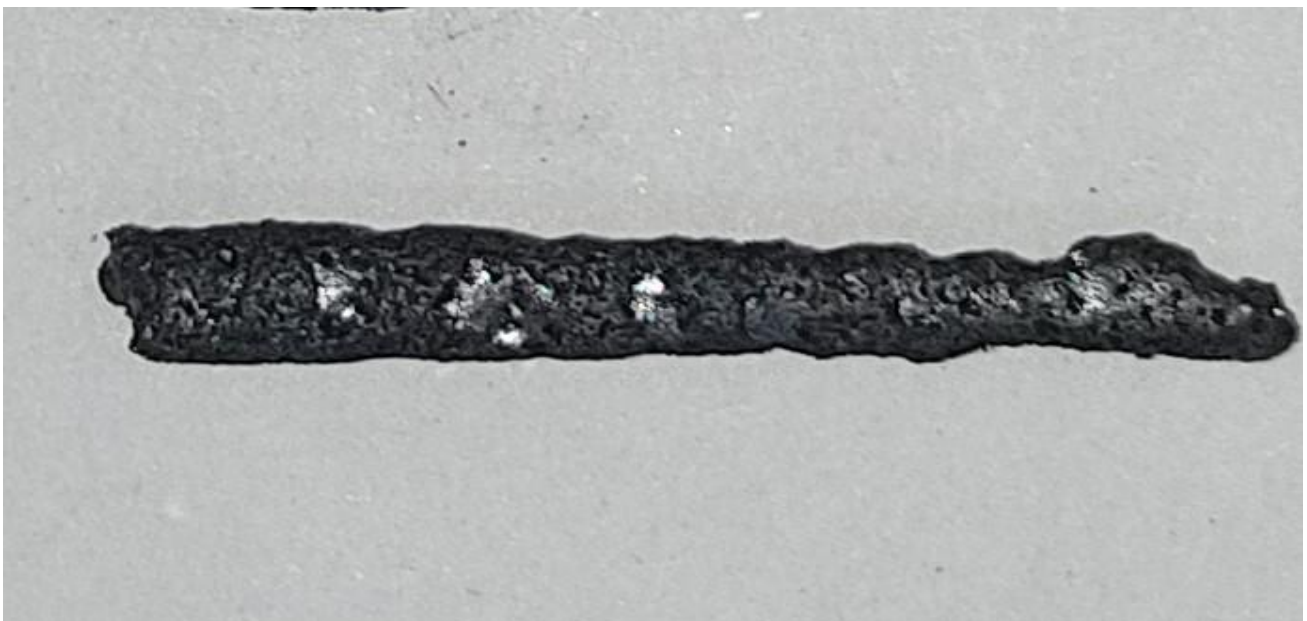
Figure 3.16. sintered iron powder (sample 3).
