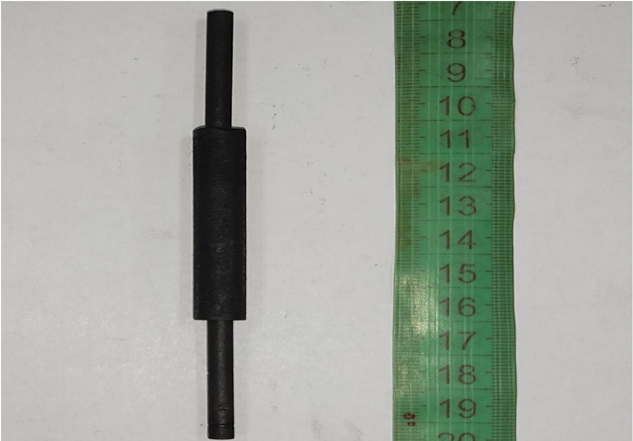
Figure 3.7. Aluminum powder pressed into a graphite die.
