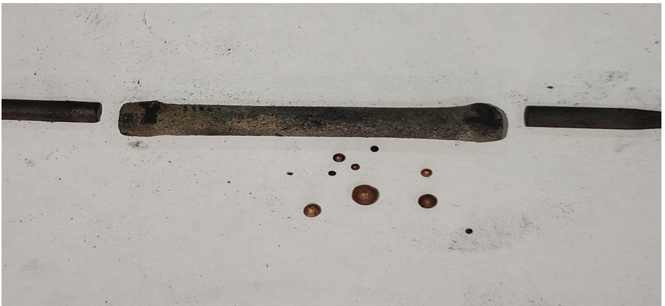
Figure 3.12. The first experiment when the copper sample exceeded the melting temperature.
