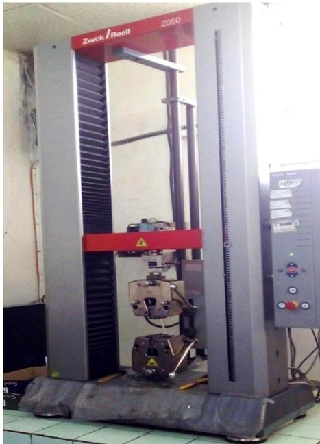
Figure II.6 : machine de traction ZWICK ROELLZ050
