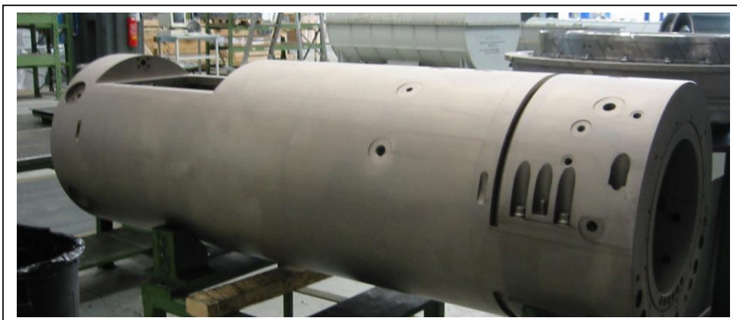
Figure.II.19 : carter-support rotor de la turbine BP
