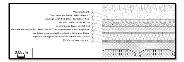
**Figure III.21** Walkable green roof detail. **Source:** (Author, June 2021)
