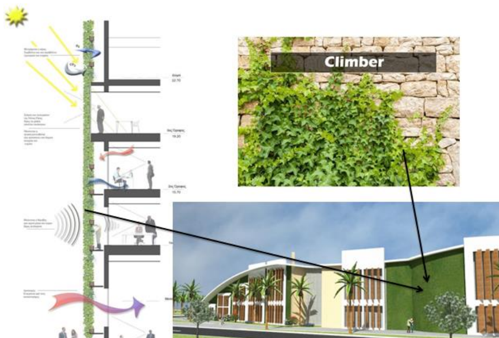
Figure 02 : the benefits of the green wall and the plant's apply on it
