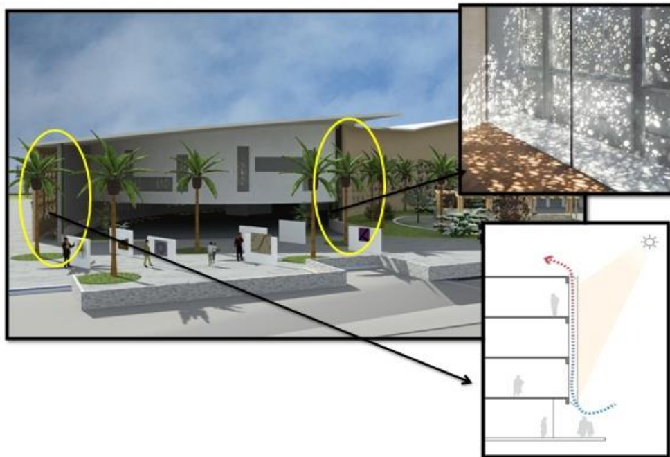
Figure 01 : details of the wall double skin.
