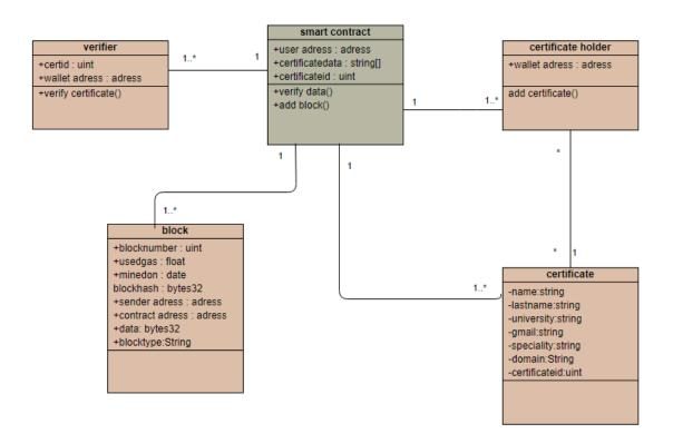
Figure 3.6: Class diagram
