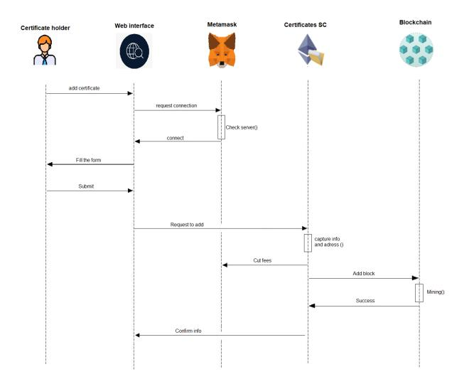
Figure 3.4: Certificate holder sequence diagram
