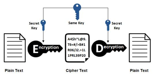
Figure 1.11: Symmetric key cryptography
