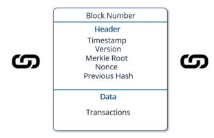
Figure 1.2: Block structure
