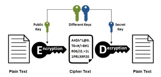
Figure 1.12: Asymmetric key cryptography
