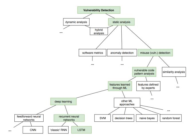
Figure 2.24: One way to structure different approaches for vulnerability detection
