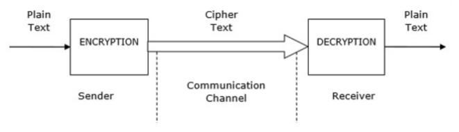
Figure 1.6: the operation of encryption[41]
