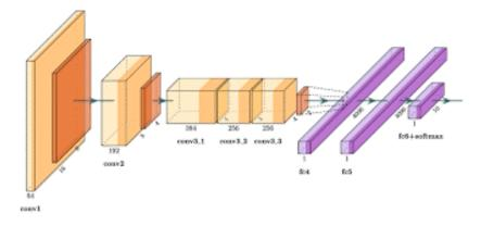
Figure 2.25: ALeXNet example.
