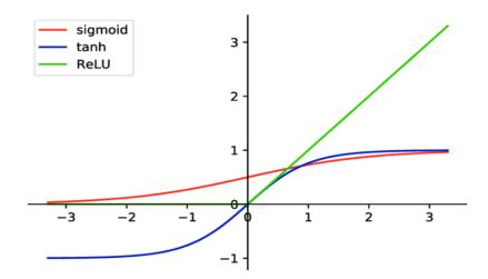
**Figure 3.4:** An illustration of Sigmoid, Tanh, and Relu function curves. Image source: [31]
