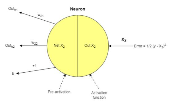
**Figure 3.8:** An example of propagating the gradient of an error through a oneneuron network. W and b are the weights and bias, Net X is the pre-activation function, Out X is the neuron's output, and Out h is the input.
