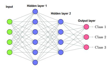
**Figure 3.7:** An example of a fully connected layers or Multi-layer perceptron (MLP)
