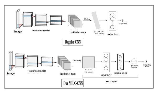
Figure 4.6: The regular CNN and the proposed MILC-CNN
