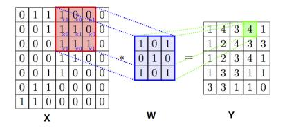
**Figure 3.2:** An example of a Convolution Operation on a single-channel image (Equation 3.1). The result of convolving the input X with a filter W is the feature maps Y.
