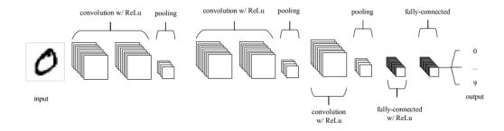
Figure 3.1: A simple CNN architecture. Image source: [56]
