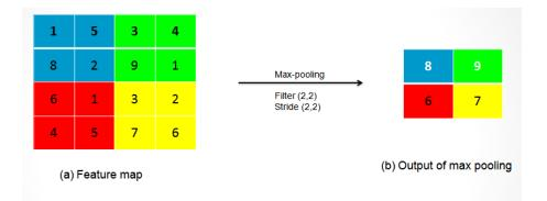
Figure 3.5: An example of max pooling
