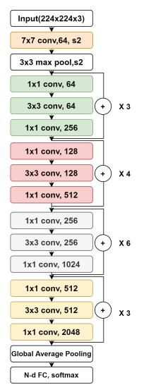
Figure 5.3: The ResNet50 architecture
