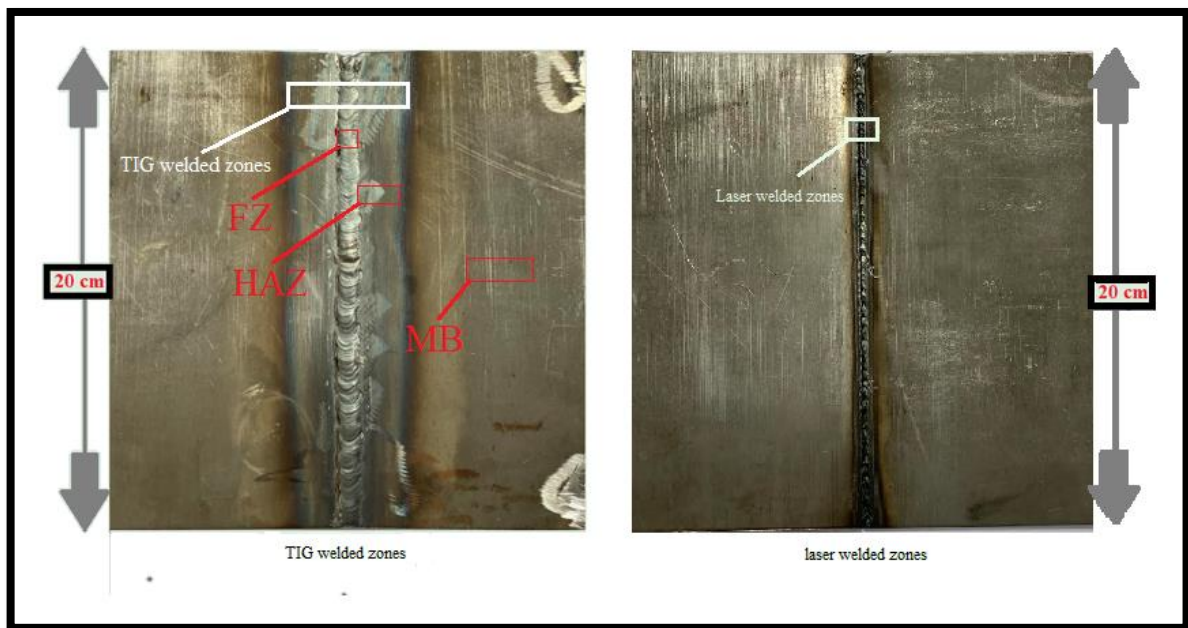
Figure III-1. Welded plats of low carbon steel by TIG and Laser welding processes.
