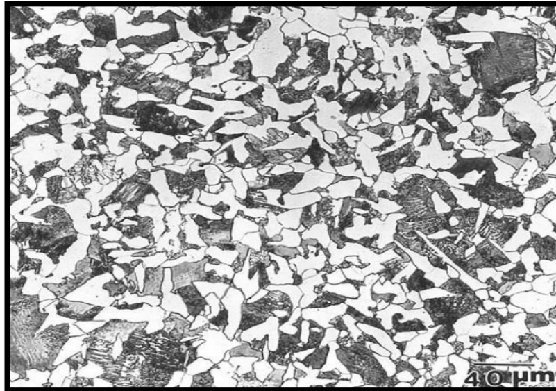
Figure II-5. Micrograph of medium-carbon steel showing ferrite grains (white etching constituent) and pearlite (dark etching constituent) [27].
