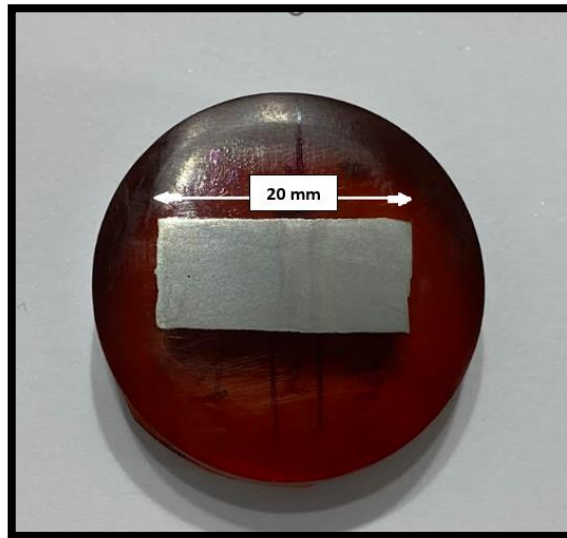
Figure III-12. Laser sample after metallographic preparation.
