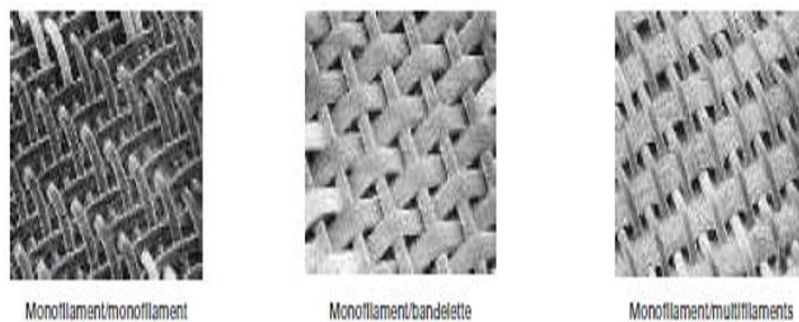
Figure II.1 : géotextiles tissés (monofilament, bandelette, multifilaments) (laurent Briançon, 2017)
