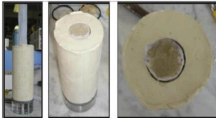
Figure II.29 : Installation de sable encacé (Najjar et al. 2010).
