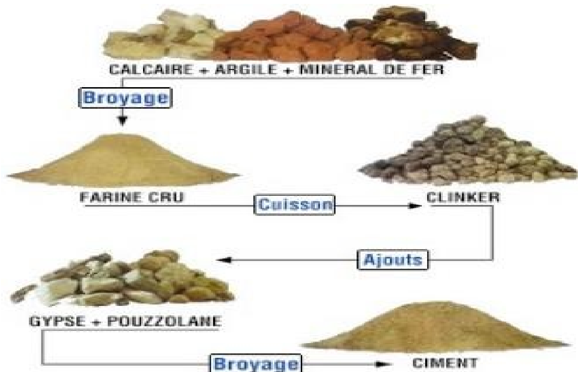
Figure I.3 : Cycle de fabrication ciment.
