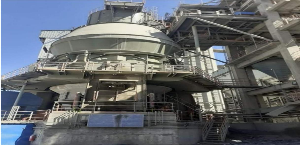
**Figure I.17 :** Broyeur ciment vertical.
