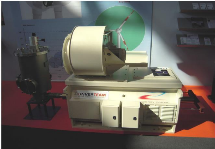
Figure II. 7 Machine ULCOMAP de 250 kW [38]
