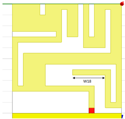
Figure 3. 8. A miniaturized monopole antenna with strip variation width W18
