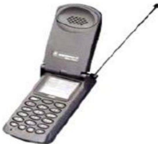
Figure 2. 13. Monopole antenna integrated in cell mobile phone [19]
