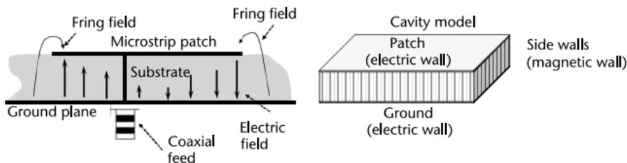
**Figure 1.3: Microstrip patch radiation mechanism and cavity model representation**
