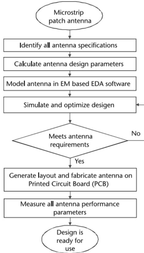
Figure 3.2 Microstrip antenna design and fabrication process
