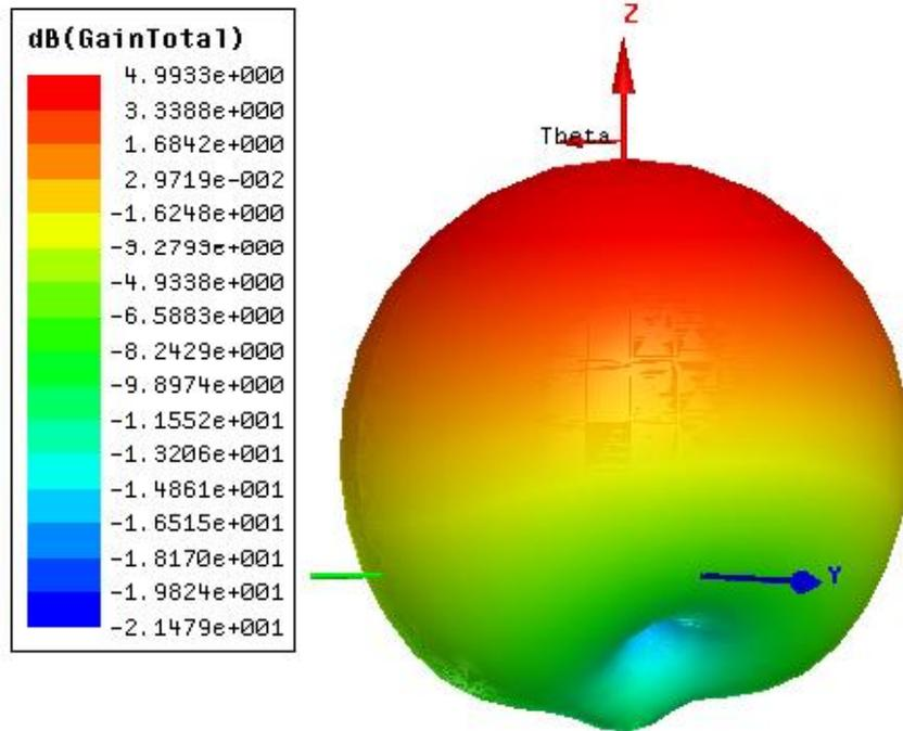
Figure 3.15:3d Polar Gain Plot
