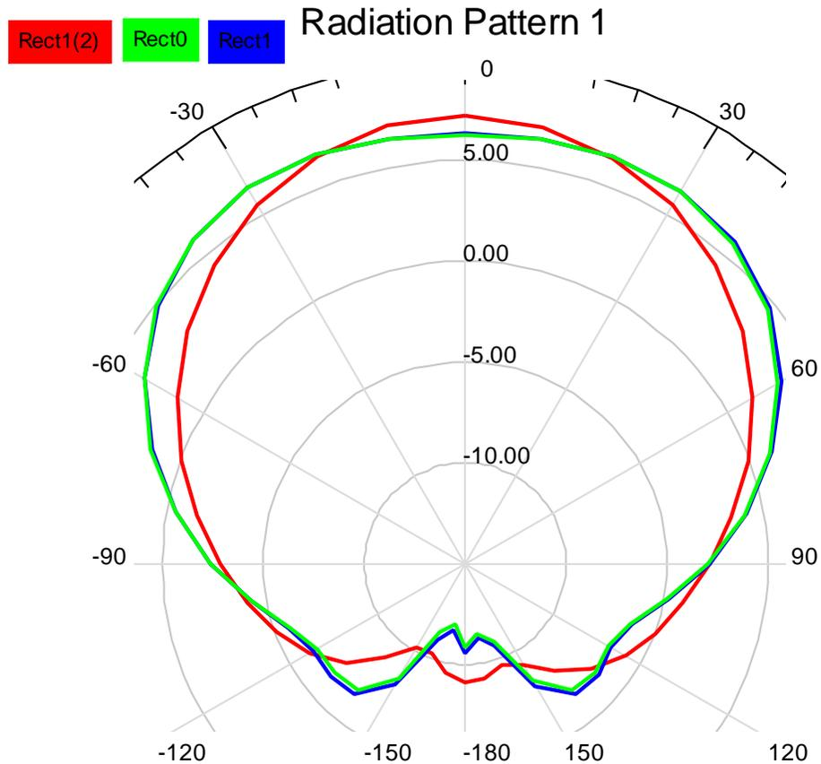
Figure 3.14: Radiation pattern comparison of Rect 0,1, and 1(2)
