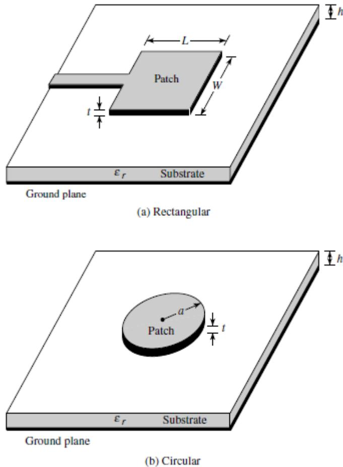
**Figure 1.1: Patch antenna most used types**
