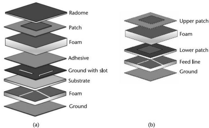
**Figure 2.9: Microstrip antenna feed mechanisms : (a) aperture-coupled antenna, and (b) proximity coupled antenna.**
