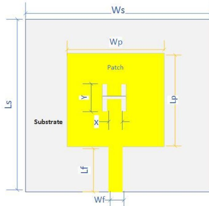
**Figure 2.10: Microstrip patch antenna with H-shape slot**
