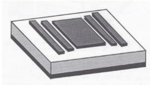
**Figure 2.12: Parasitic microstrip antenna patch**
