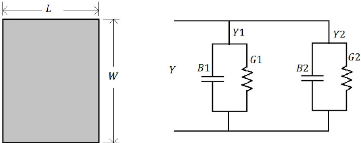
**Figure 1.5: Rectangular patch and its transmission model equivalent**
