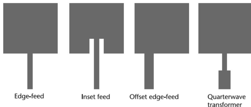
Figure 2.7 Different feeding mechanisms in a microstrip patch antenna
