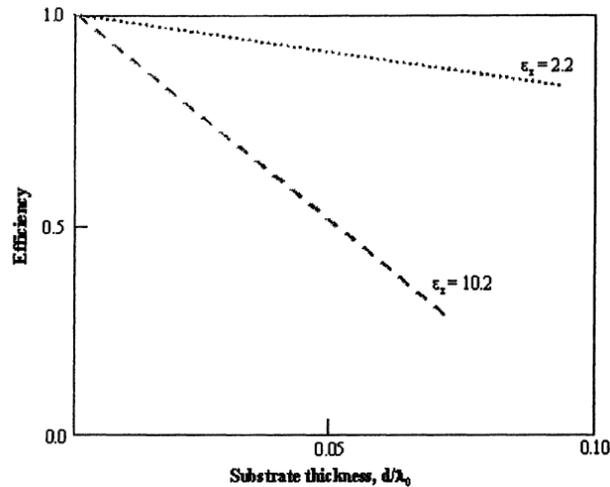
**Figure 2.5: Performance trends of single-layered patch antennas: (a) impedance bandwidth; (b) directivity; (c) surface wave efficiency**
