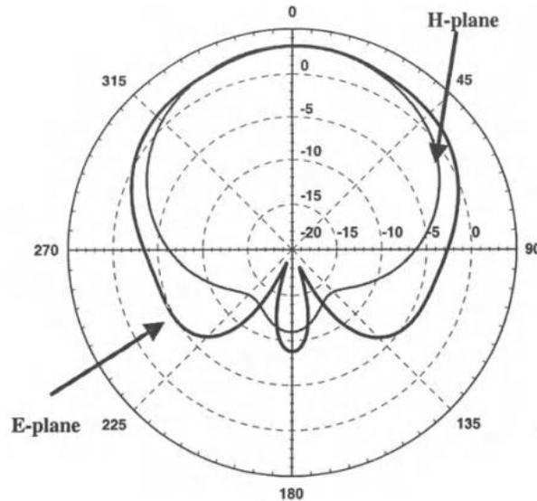
**Figure 2.6: Radiation Pattern of a Microstrip Patch Antenna (11)**
