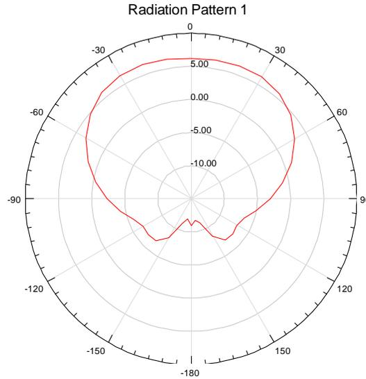
**Figure 3.7: Radiation Pattern Last Adaptive Frequency 10GHz with Phi=0deg**
