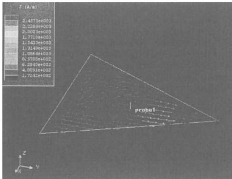
**Figure 2.3: Typical Fields Excited on a Triangular Patch Antenna**
