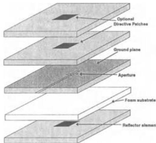
**Figure 2.16: Geometry of Aperture Coupled Microstrip Antenna with Reflector Element**
