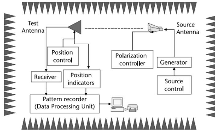
Figure 2.18: Antenna radiation pattern measurement setup in an anechoic chamber.
