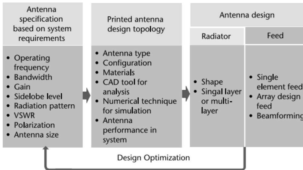
Figure 3.1 Microstrip patch antenna design flow
