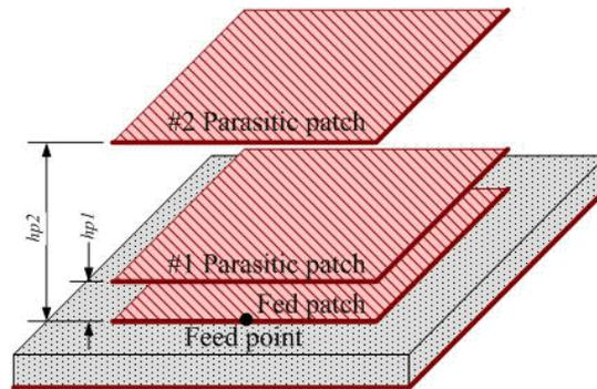
**Figure 2.14: 3-Element Stacked Microstrip Antenna with Wide-Band and High-Gain Performances**
