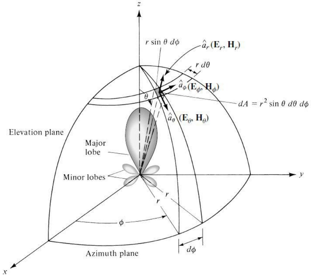
Figure 1.4 : Radiation pattern graphical representation (1)
