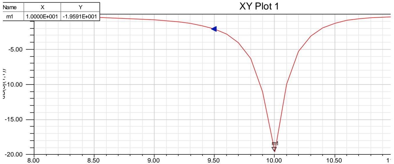
**Figure 3.5:S-Parameter S11 in the function of frequency**
