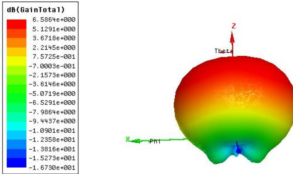
**Figure 3.8:3D Gain Polar Plot**
