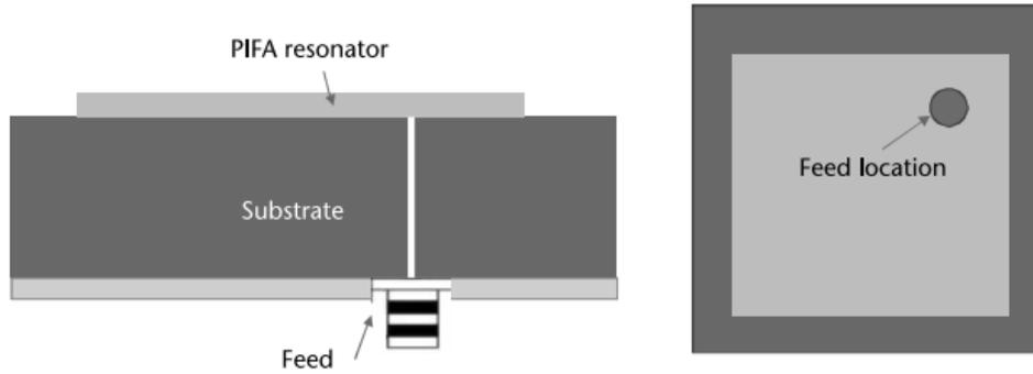
**Figure 2.8 Coaxial-fed microstrip patch antenna (side and top view)**
