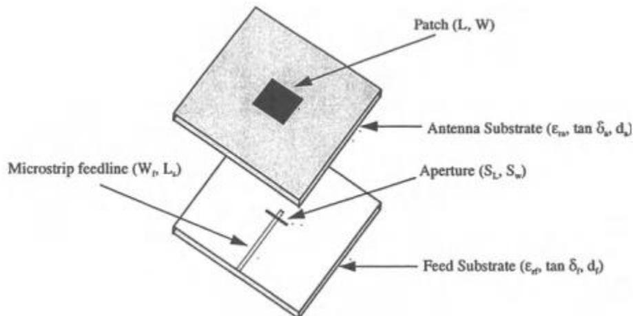
**Figure 2.15: Large Slot Aperture Coupled Patch Antenna**
