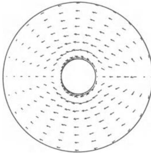
**Figure 2.4: Typical Currents/Fields Excited on an Annular Ring Patch**
