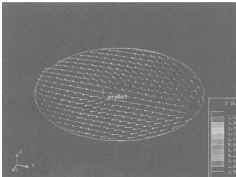
**Figure 2.2: Typical Fields Excited on a Circular Patch Antenna**
