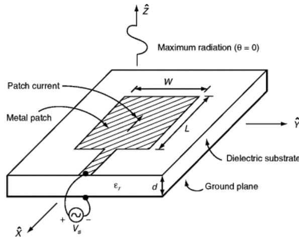
**Figure 2.1: Geometry of a Rectangular Microstrip Antenna.**
