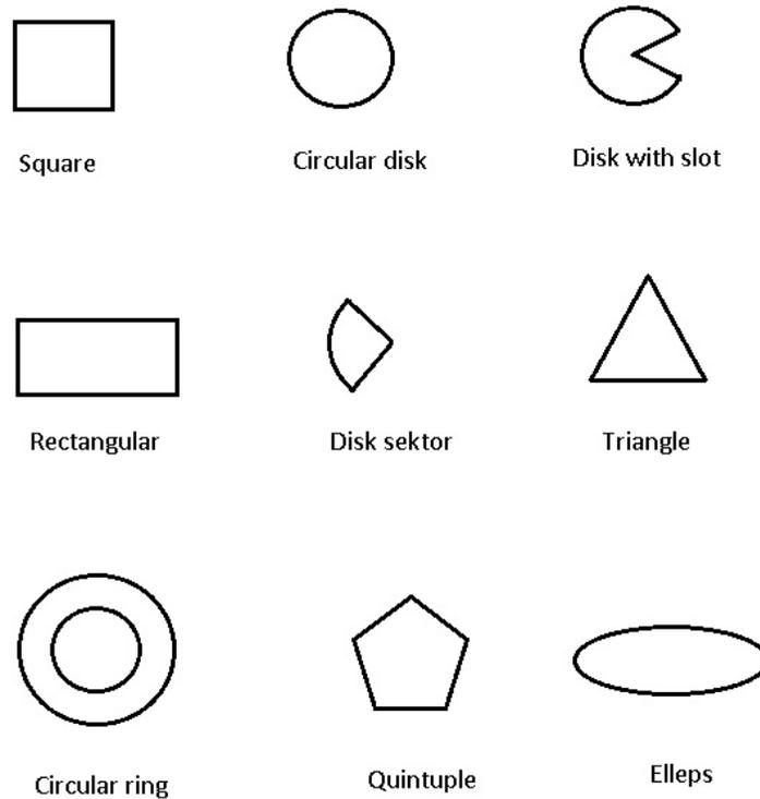
**Figure 1.2: Antenna patch types**
