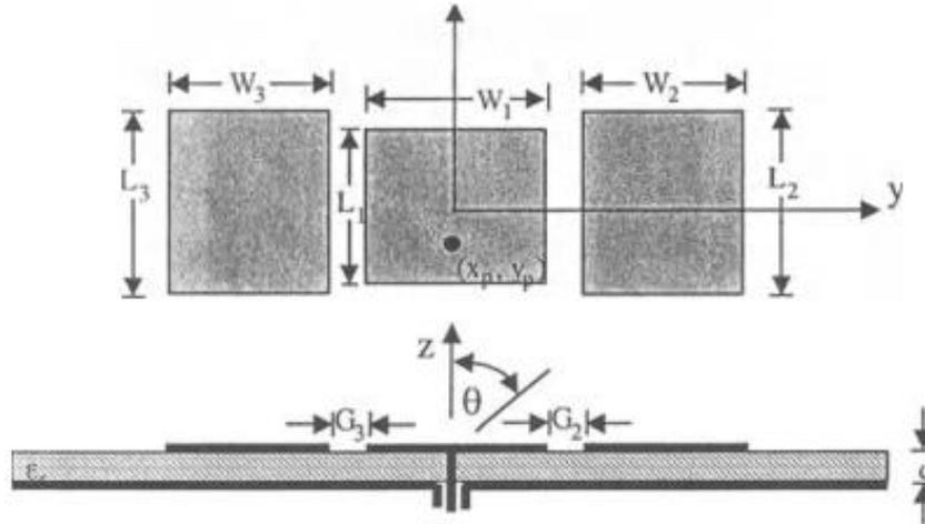
**Figure 2.11: Horizontal Parasitically Coupled Patches**
