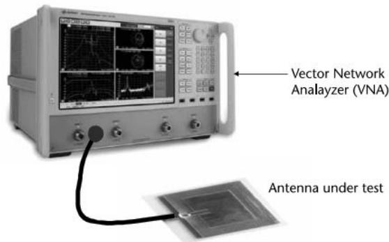
Figure 2.19: Antenna S-parameter and input impedance measurement setup using a vector network analyzer
