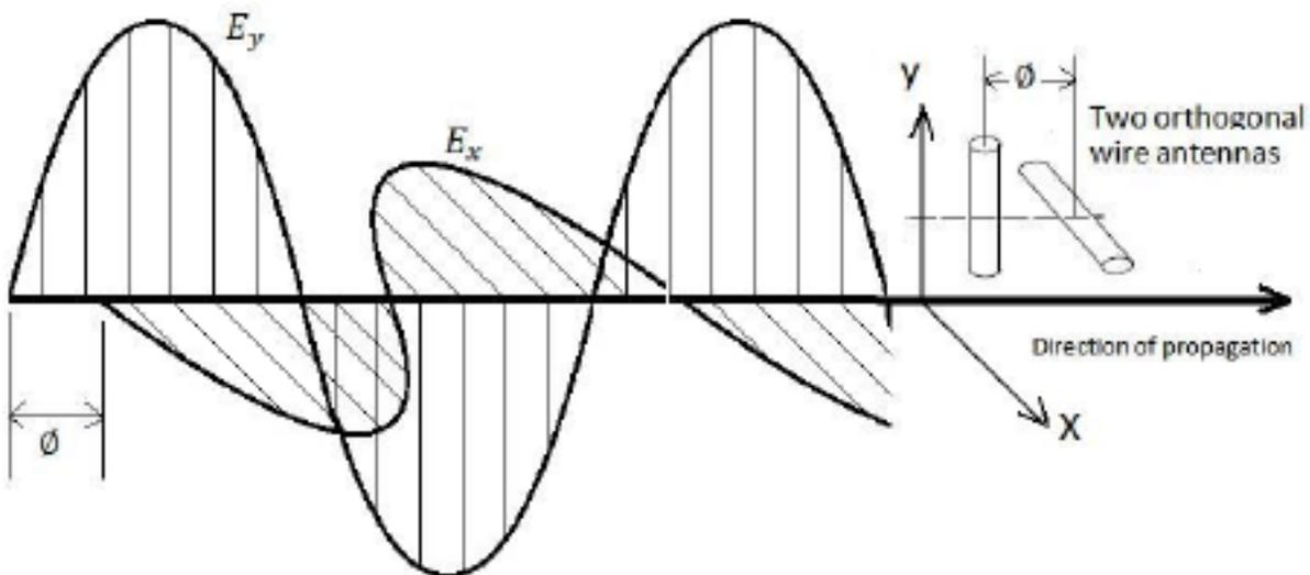
**Figure 1.7: Polarization of electromagnetic wave**
