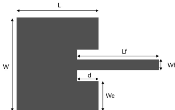
**Figure 3.3: Inset fed rectangular microstrip antenna design**
