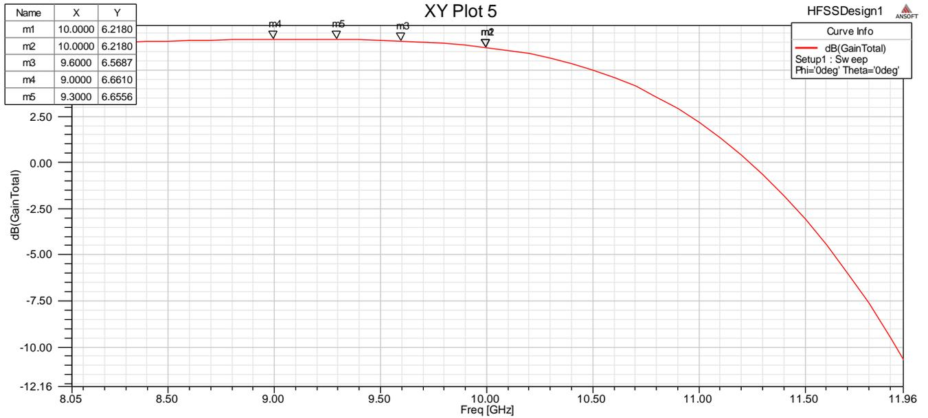
Figure 3.9: the Gain variation in terms of the Frequency
