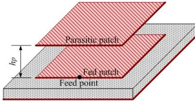
**Figure 2.13: Stacked Microstrip Antenna**
