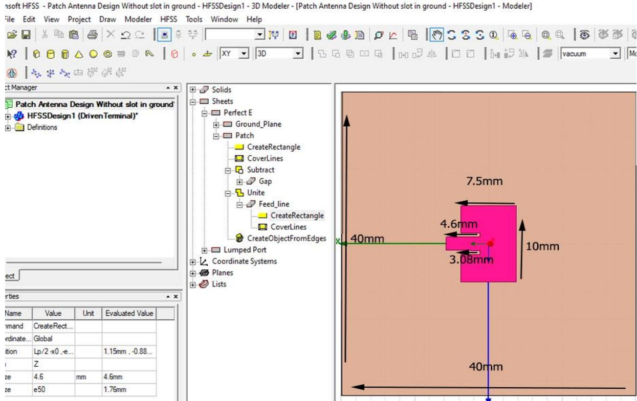
**Figure 3.4: Patch antenna and substrate dimensions on Hfss**
