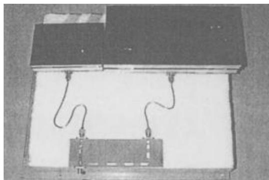
**Figure 2.17: Photograph of Ultra-wideband Printed Antenna**
