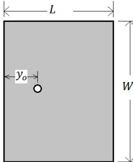
**Figure 1.6: Dimensions of patch**
