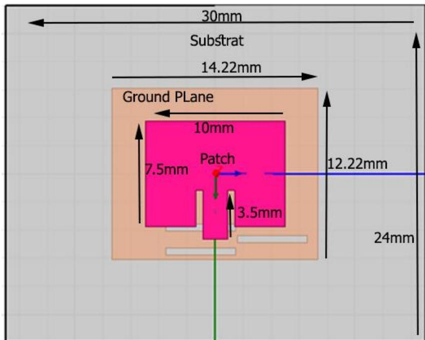
Figure 3.12: Final Form of the rectangular microstrip antenna
