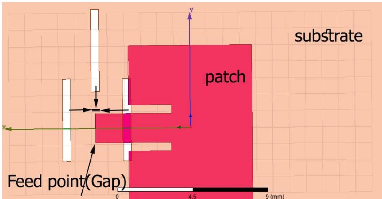
Figure 3.11: microstrip antenna with 3 slots in the ground plane
