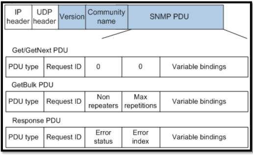
Figure II 13 : Format of SNMPv1 and SNMPv2c get packets
