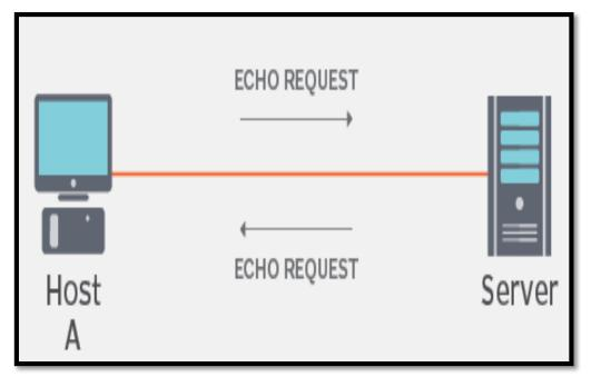
Figure II 15 : Echo-request and echo-reply in ICMP
