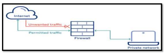
Figure II 24 : Diagram of firewall in network
