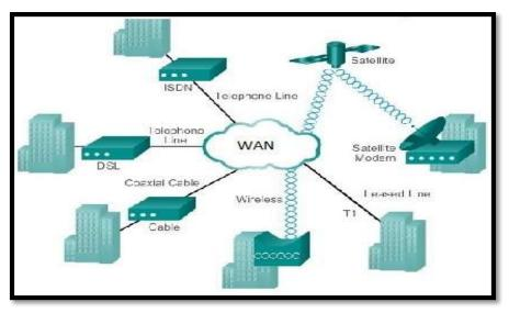
Figure I 5 : Diagram of WWAN
