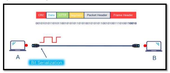
Figure I 12 : Diagram showing the physical layer
