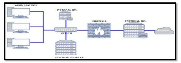
Figure II 26 : Intrusion Detection System model
