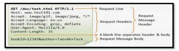
Figure II 2 : Structure of HTTP request massages
