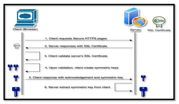
Figure II 21 : Diagram of how HTTPS works
