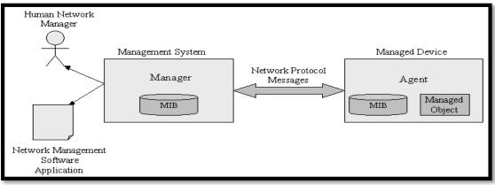
Figure II 10 : Diagram of SNMP runtime components
