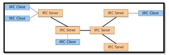
Figure II 8 : Multi-server IRC architecture
