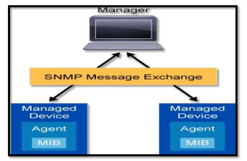
Figure II 9 : Diagram of SNMP between agents and manager
