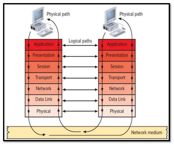
Figure I 11 : Flow of data through the OSI model
