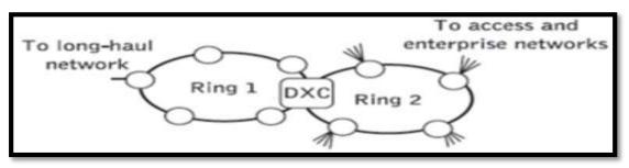
Figure I 8 : The structure of a metroplitan network
