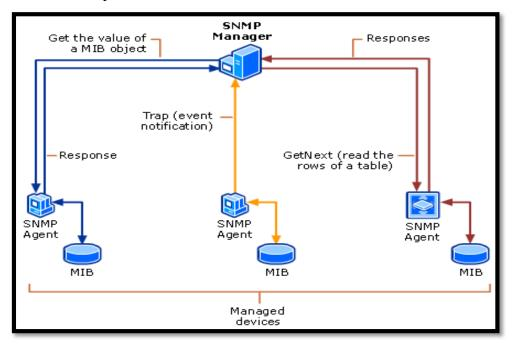
Figure II 12 : Diagram of how SNMP works
