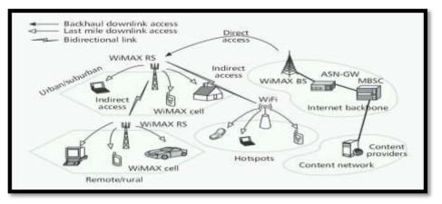
Figure I 10 : Diagram showing multicast/broadcast WiMAX system architecture
