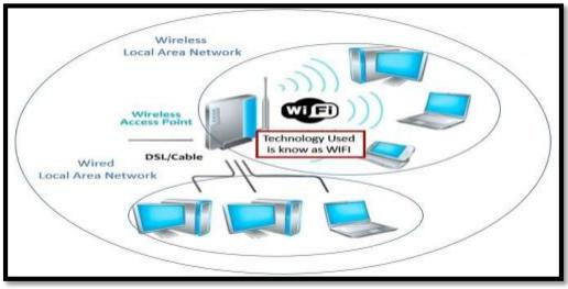
Figure I 3 : Diagram of wired and wireless LAN
