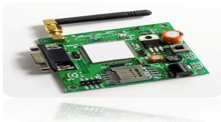
FIGURE III.13. GSM 900 Board
