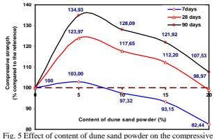
Fig. 5 Effect of content of dune sand powder on the compressist strength ( $F2 = 4000 \text{ cm}^2/\text{g}, w/b = 0.25$ )
