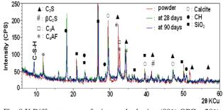
Fig. 8 X Diffractograms of mixtures hydration (80% OPC + 20% DSP) as a function of time
