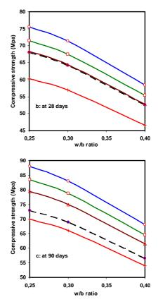
Fig. 2 Variation in compressive strength as a function of time and w/b ratio ( $F_1 = 3000 \text{ cm}^2/\text{g}$ )
