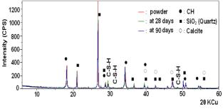
Fig. 7 X Diffractograms of mixtures hydration (50% Pure Lime + 50% DSP) as a function of time
