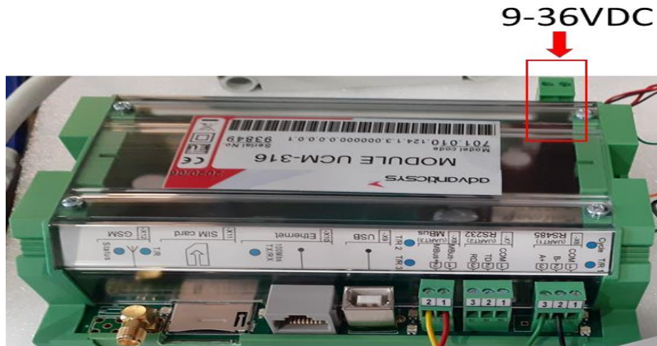
Figure III 25 : UCM-316 power supply input.
