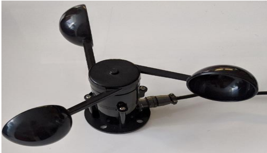
Figure III 3: Wind speed sensor
