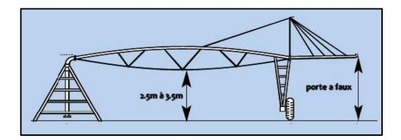
Figure 4 Diagram represents the dimensions of a pivot
