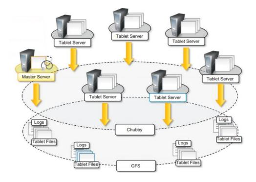
Figure II.10: The architecture of the Bigtable.
