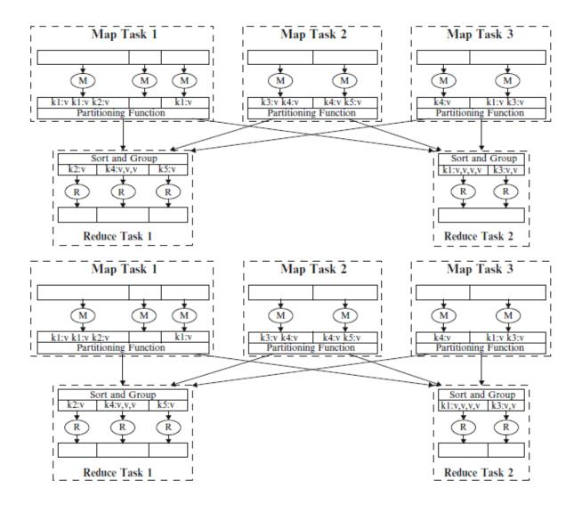
Figure II.6: Distributed Processing using Map Reduce.
