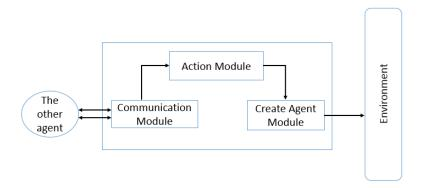
Figure V.8: Concrete Architecture of the Planning Agent
