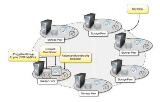
Figure II.9: The architecture of Amazon Dynamo.
