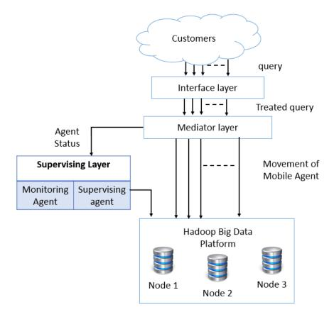
Figure V.4: Architecture illustration of the monitoring phase
