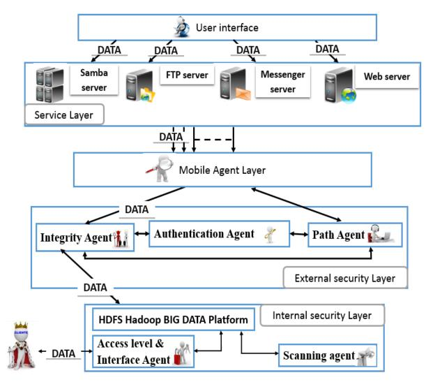
Figure IV.1: Proposed Architecture using Multi-Agent System
