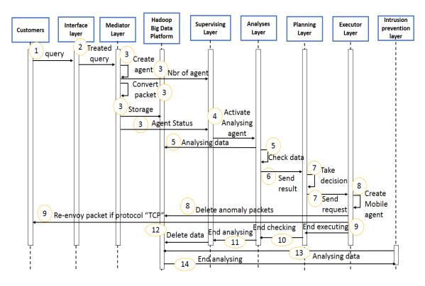
Figure V.9: Sequence Diagram of SLA-IDS
