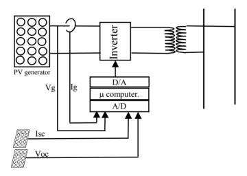
Figure 10 : Grid connected PV system
