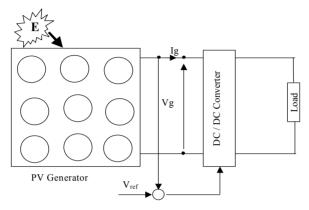
Figure 7 : MPPT without temperature compensation
