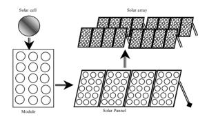
Figure 2 : PV generator hierarchy
