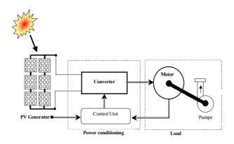
Figure1: Schematics of a photovoltaic pumping system
