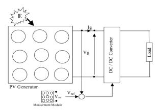
Figure 8: MPPT with temperature compensation
