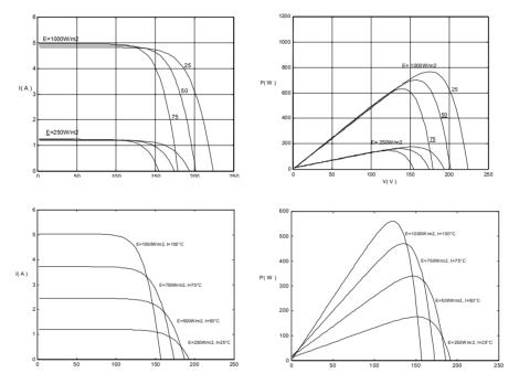
Figure 4 : Photovoltaic generator characteristics as a function of: - a-b: Solar insolation (250-1000 W/m<sup>2</sup>) and temperature (25,50 and 75° C)c-d: Solar insolation and temperature simultaneously
