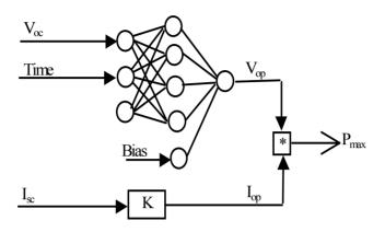
Figure 11 : Configuration of Neural Network
