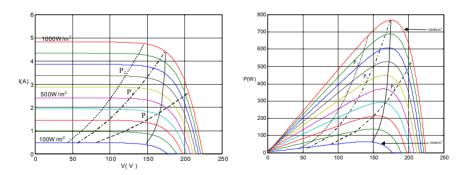
Figure 5: I-V and P-V characteristics of a PV pumping system, T=25°Ca) I-V characteristicsb) P-V characteristicsLoad CharacteristicsMaximum power locus
