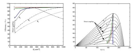
Figure 9 : System power efficiency as a function of solar insolation 1: True MPPT 2:  $V_{ref} = %V_{co}$  3:  $V_{ref} = Cte$  $P_1, P_2, P_3$ : Direct Coupling
