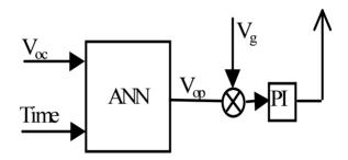
Figure 12 : Block diagram for optimal voltage identification
