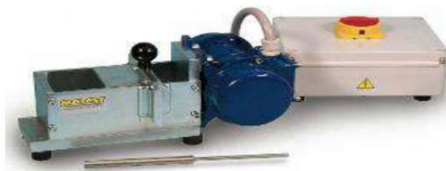
Figure II.7. Apparatus for workability measurement (LCL workabilimètre).
