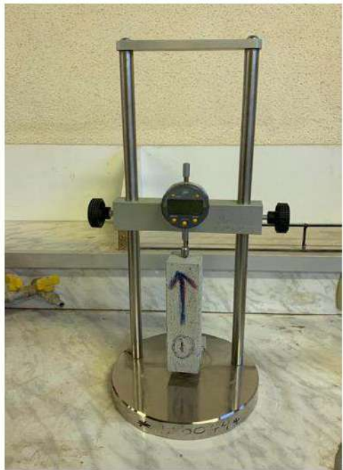
Figure II.12. Shrinkage test method.
