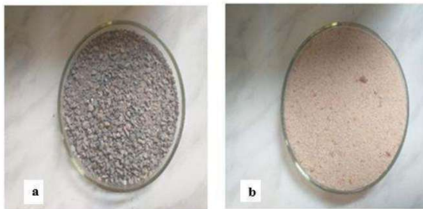
Figure II.1. (a) Crushed sand and (b) river sand.
