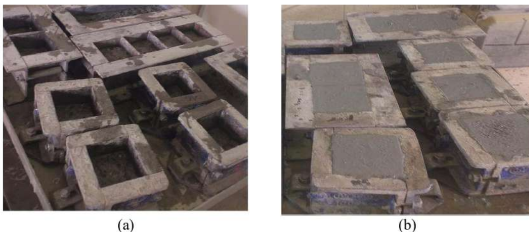
Figure.II.19. (a) Substrate fixing molds for repair materials, and (b) apply repair materials to concrete Substrates.
