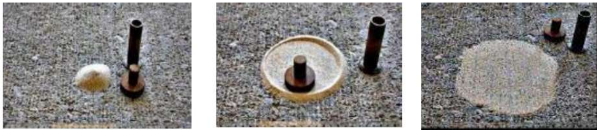
Figure I.21. Mechanism for conducting a sand patch test (Courard et al., 2014; López-Carreño et al., 2017).
