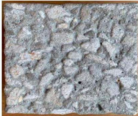
(c) surface of the substrate using sandblasting (SB)
