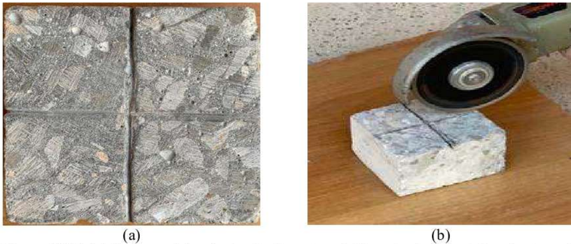
Figure.II.18. (a) Surface of the obtained substrate and (b) method of obtaining the treated surface using a stone rocket.
