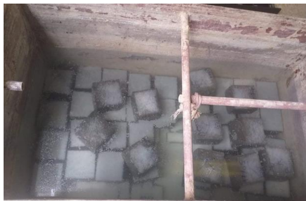
Figure II.12. Curing of concrete specimens in water for 28 days.
