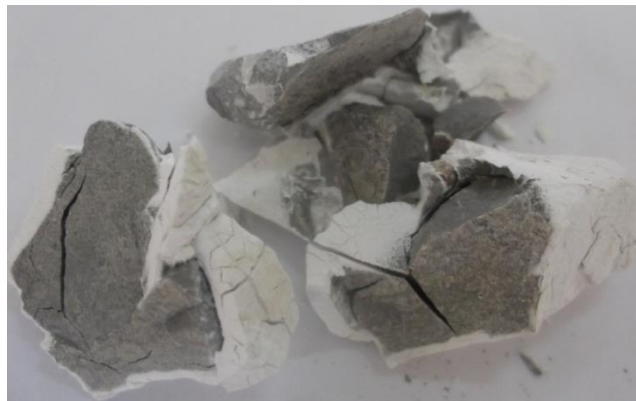
Figure I.12. Cracking of calcareous aggregate immediately after heating to 900°C [Hachemi, 2015].
