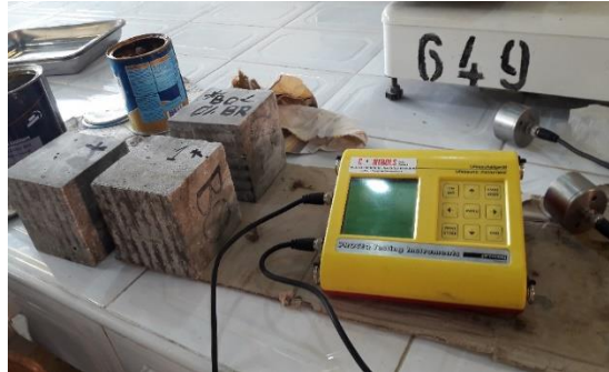
Figure II.18. UPV measuring device.
