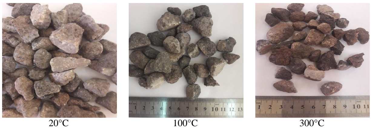
Figure III.11. Pictures of coarse RBA-1 before and after exposure to different temperatures.
