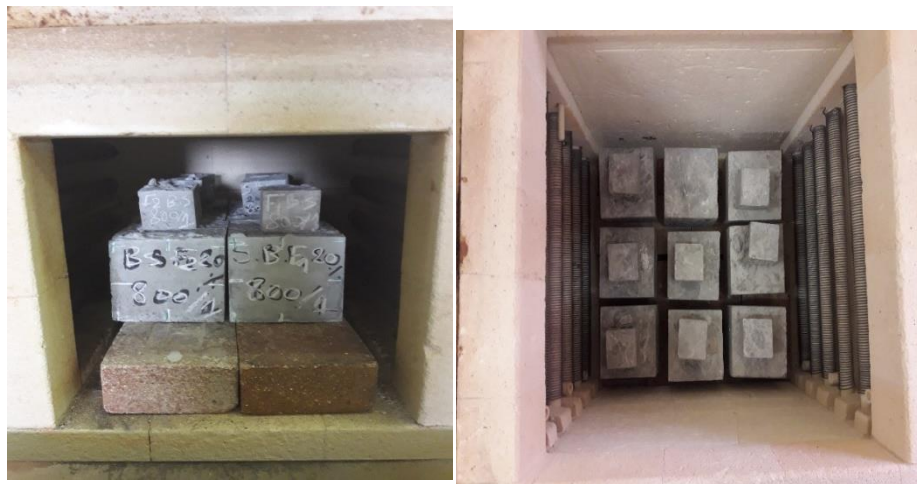
Figure II.14. View of concrete specimens inside the furnace.
