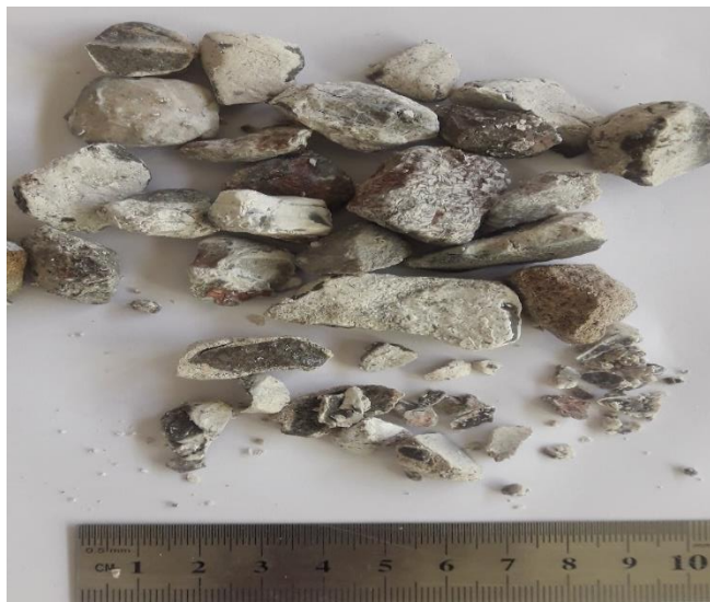
Figure III.10. Coarse NA after a heating to 900°C and immersing in water for 24 h.
