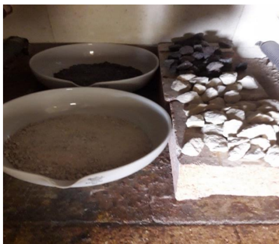
Figure II.23. View of aggregate inside furnace.
