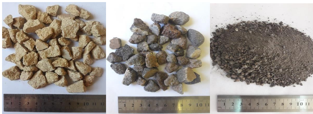
(a) (b) (c) Figure II.4. Refractory brick aggregate after crushing: (a) coarse RBA-1 (b) coarse RBA-2 (c) fine RBA-2.
