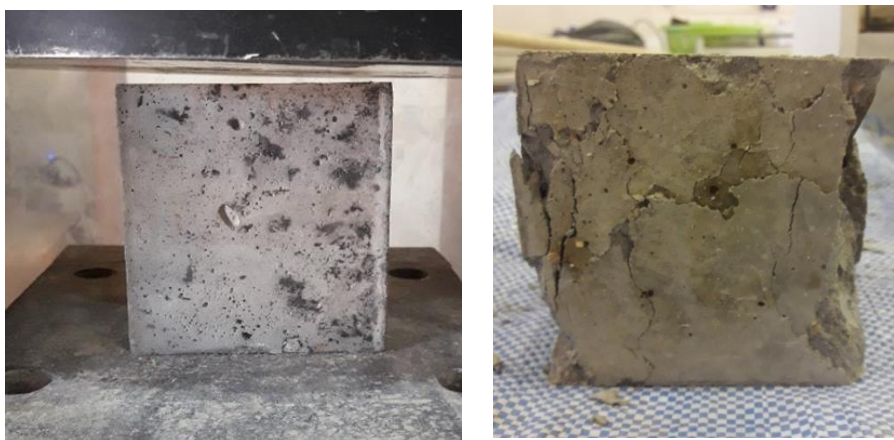
Figure II.17. Test sample placed on the hydraulic press to determine the compressive strength.
