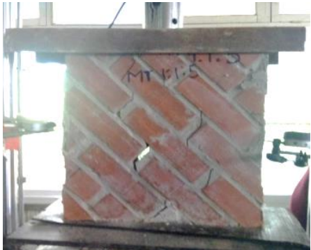
(b) Failure modes of unstrengthened masonry panels 45° (MTB)
