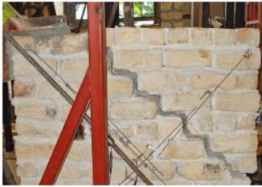
Figure 2.25 diagonal crack in a Wallette and debonding of CFRP plate [51]
