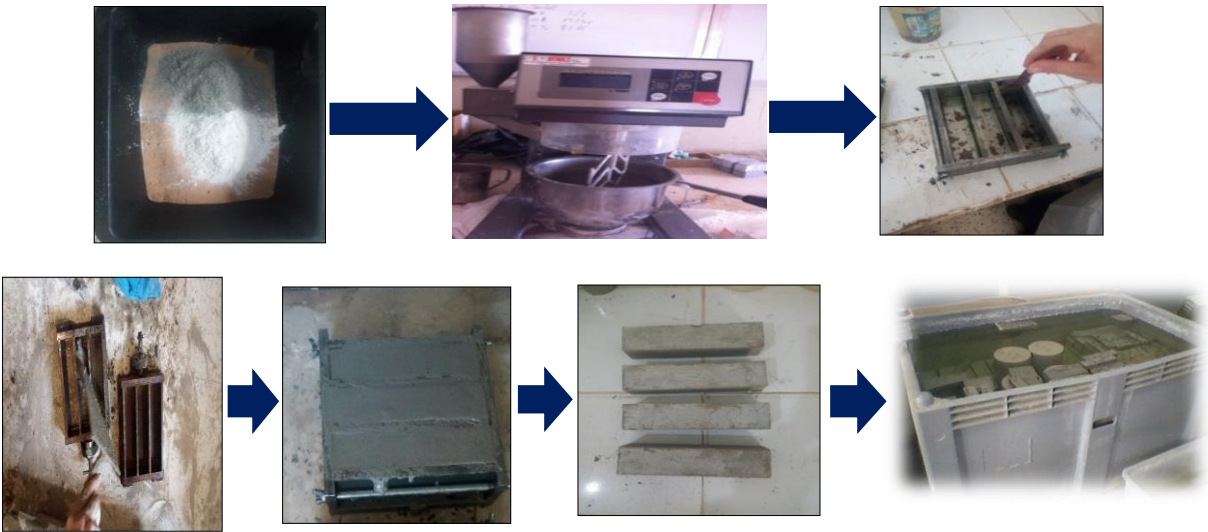
Figure 3.6 Preparation and storage of prismatic test pieces of dimensions 40x40x160 mm
