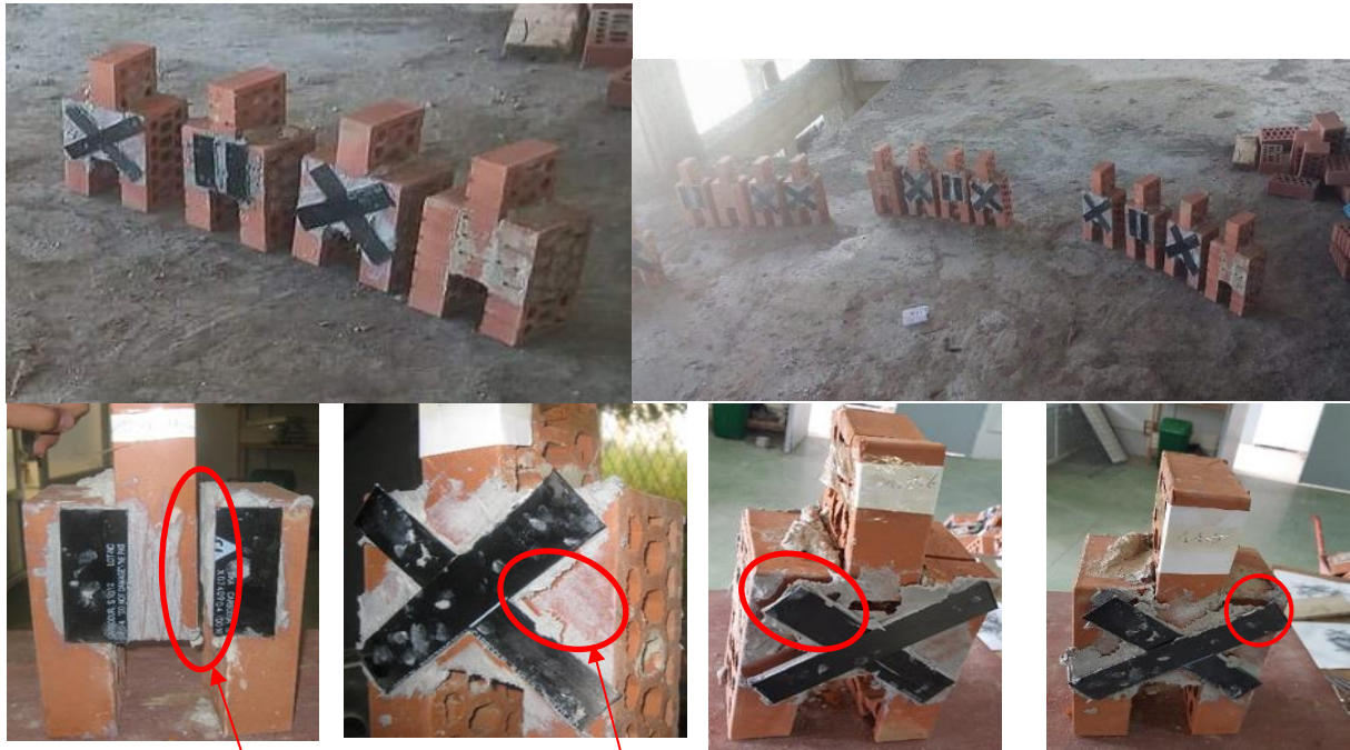
Failure with sliding at the interface and cracking of mortar joint
