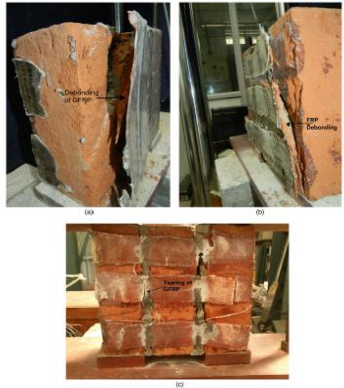
Figure 2.42 Failure patterns of triplet specimen with CFRP composite:(a) and (b) debonding failure, (c) tensile rupture failure [62]
