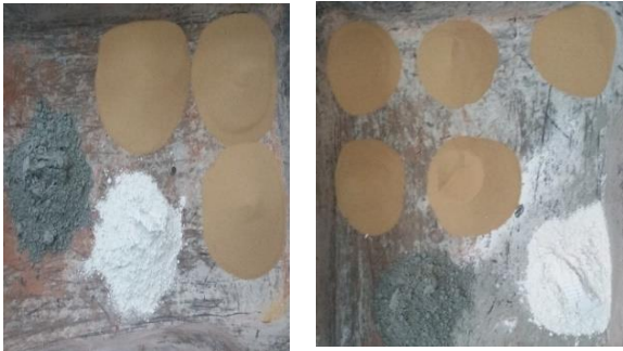
Figure 3.5 The cement-lime-sand dosage for the preparation of mortar
