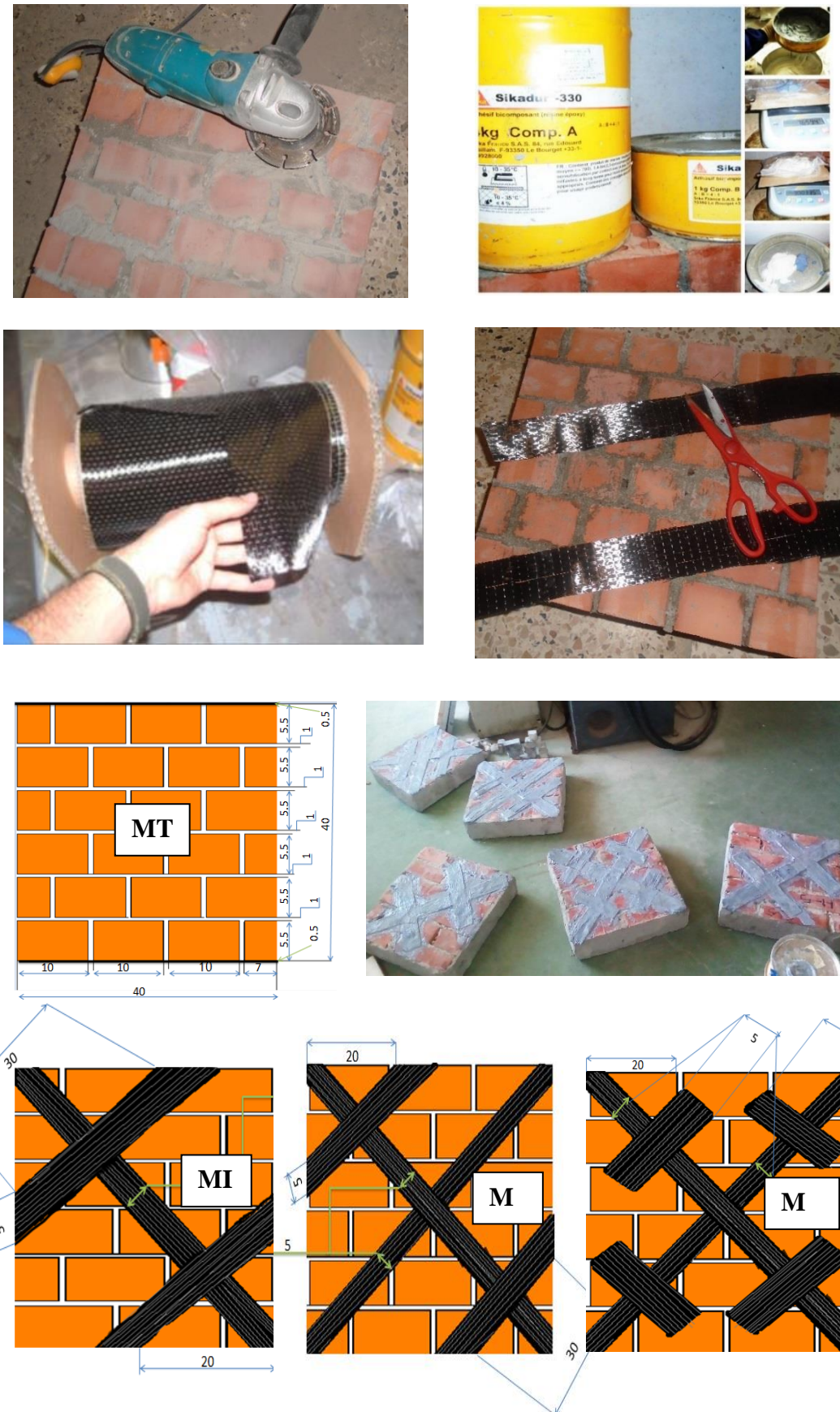
Figure 3.16 Specimen preparations and configuration of reinforcing for masonry panels
