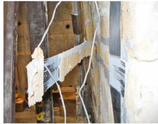
Figure 2.25 diagonal crack in a Wallette and debonding of CFRP plate [51]
