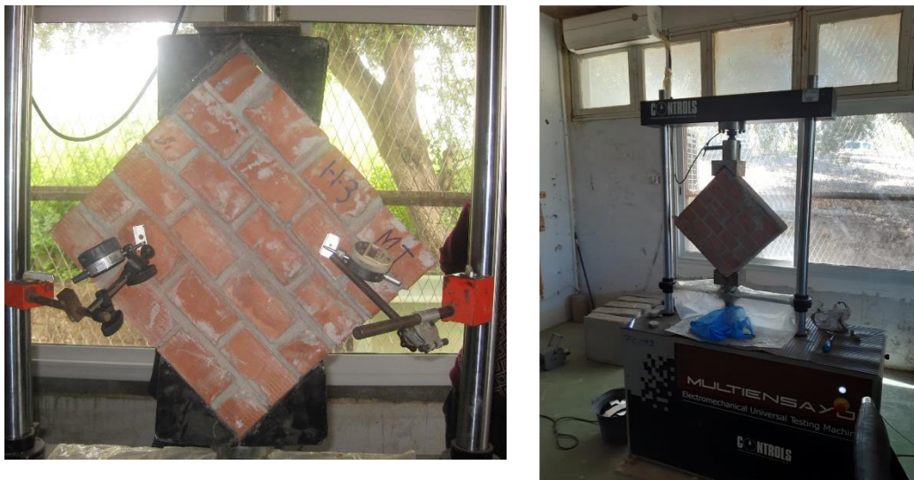
Figure 3.17 Experimental setup of unreinforced masonry panels tested in diagonal compression
