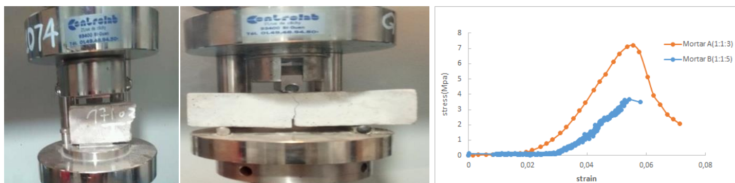
Figure 3.7 Test Mortar and Compressive stress-strain response of different type of mortar
