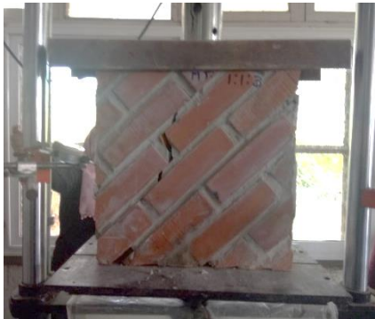
(a) Failure modes of unstrengthened masonry panels 45° (MTA)
