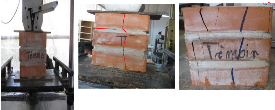
Figure 3.8 test arrangement and crack pattern of masonry prism
