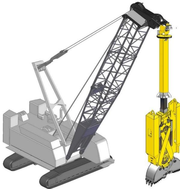
Figure 1.12 Trench excavation by the MHL method. Ou, C. Y. (2014). Deep excavation: Theory and practice. Crc Press.
