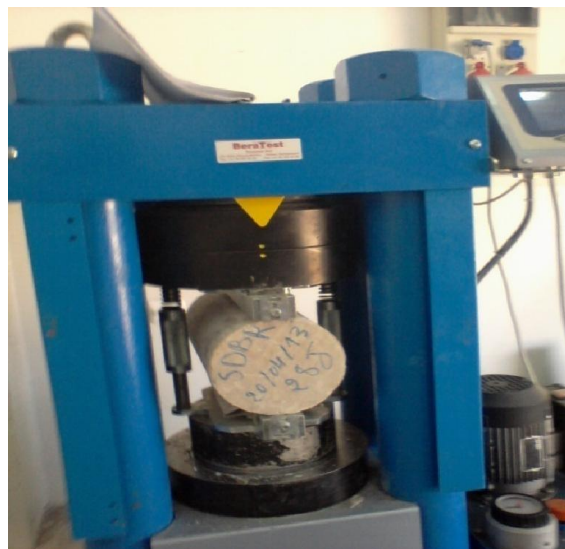
Photo 3-20: Essai de fendage
