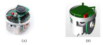
FIGURE 4.4: (A) The real e-puck robot. (B) a CAD model for the e-puck robot.
