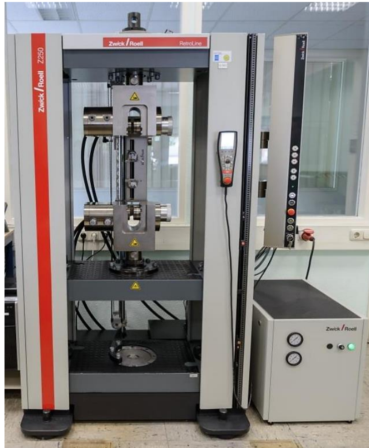
Figure II.11- Machine de traction de type Zwick Roell Z250.
