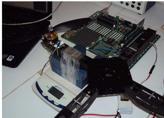
Figure 6.4: Trust factor experiment testbed.
