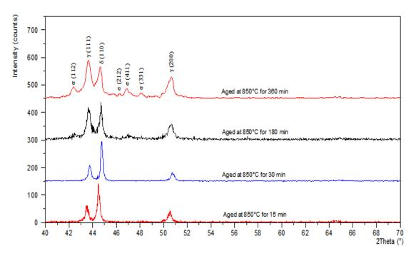
Figure III. 12: X-Ray diffraction patterns of samples aged at 850°C.
