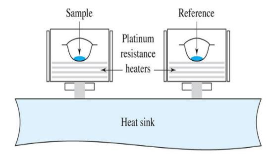
**Figure II.10 :**Schematic illustration of power compensation DSC [KOD 14].
