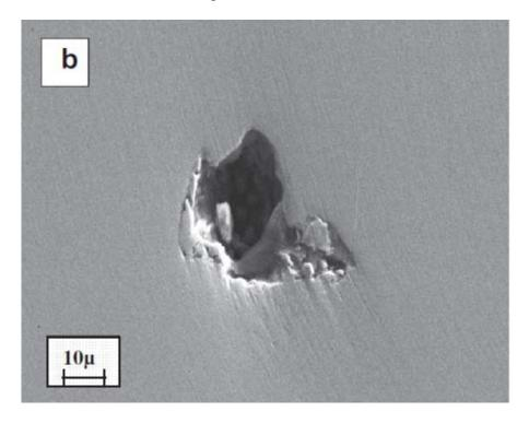
**Figure A.8:** Pit morphology of DSS 2205 after corrosion test in 0.1 M NaCl + 0.01 M  $MoO_4^{-2}$  at 80 °C [EGH 11].
