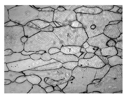
**Figure A.1:** Optical micrograph of DSS at solution treated condition, after electrochemical etching is with a 32 N KOH [BAD 14].
