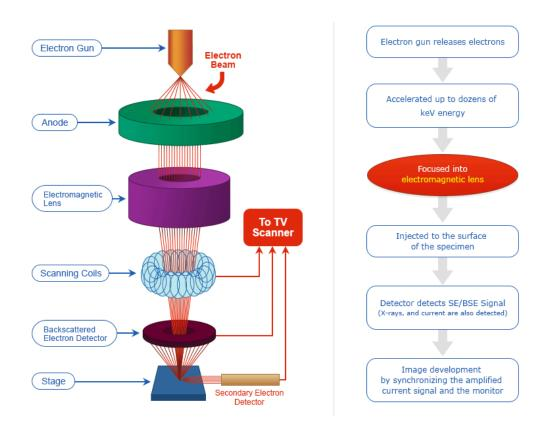
**Figure II.9:** Schematic diagram of major components of SEM [NAN 20].
