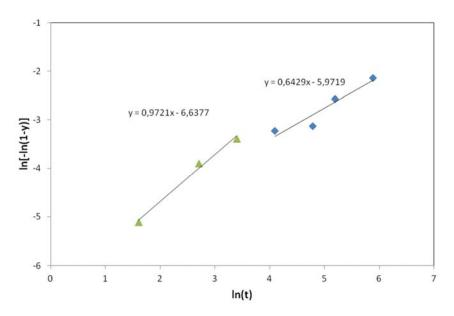
**Figure III. 8:** Application of the classical JMA model for sigma phase formation mechanism in at 850 °C.
