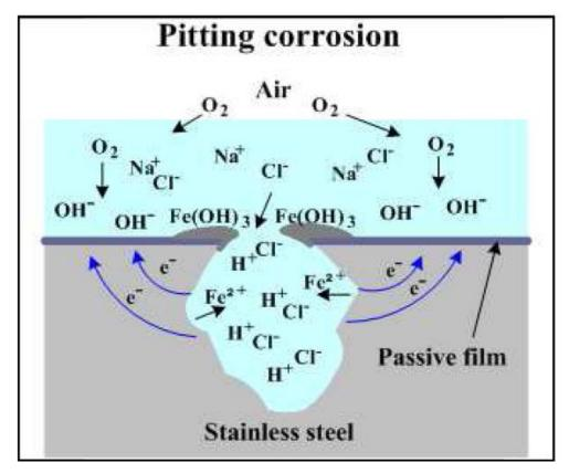
**Figure I.19:** typical schematic for pitting corrosion process [SAU 11].
