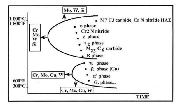
**Figure I.6:** Schematic TTP, time-to-precipitation, diagram for duplex stainless steels with secondary phases and influence of alloying elements[CHA 91]
