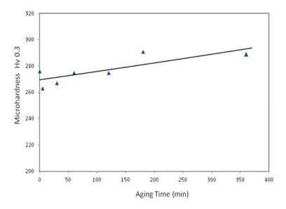
**Figure III. 25:** Microhardness evolution as a function of aging time at 850°C for the studied DSS (UNS S31803).
