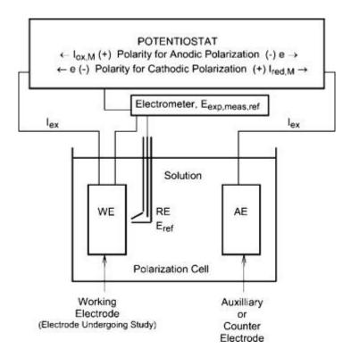
**Figure II. 15:** Schematic of the electrochemical cell used for corrosion testing [BUC 12].
