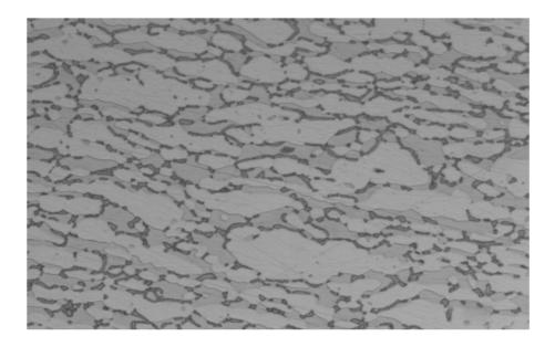
**Figure A.3:** Micro-section showing sigma phase precipitates in a super DSS fitting. (electrolytically etched in oxalic acid then KOH; X500) [ROG 12].
