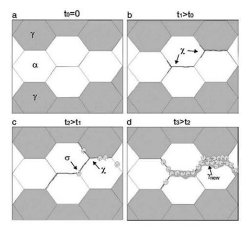
Figure I.11: Chi phase precipitation in DSS [ESC 09].
