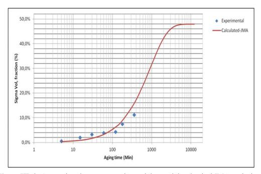
**Figure III. 9:** Comparison between experimental data and the classical JMA analysis of sigma volume fraction during aging at 850°C.
