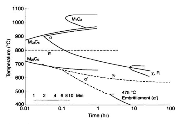
Figure I.14: Time-Temperature Transformation diagram for alloy S32404 [GUN 03].
