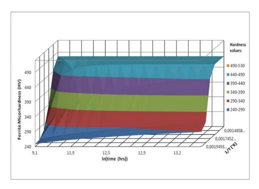
Figure III.17: Predicted Microhardness surface for aged 2205 DSS grade.
