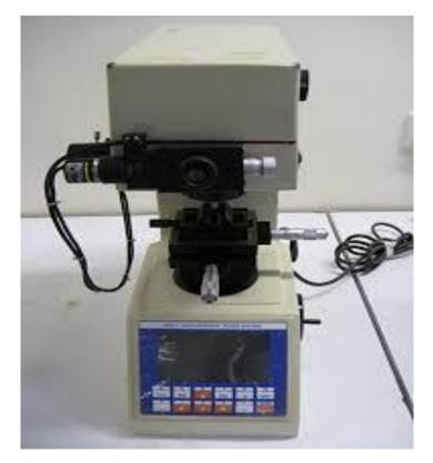
Figure II.6: Microhardness apparatus.
