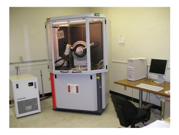
Figure II.8: Bruker D8- Advanced diffractometer.
