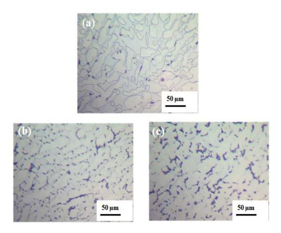
**Figure III. 6:** Optical micrographs showing the aged specimens at 850°C for (a) 5 min, (b) 60min and (c) 360min.
