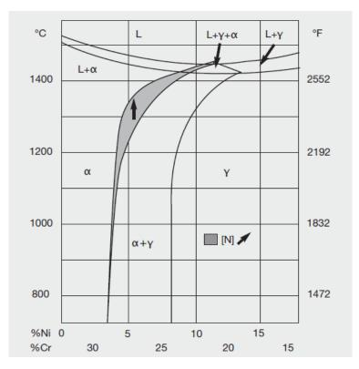
**Figure I.10:** Section through the Fe-Cr-Ni ternary phase diagram at 68% iron (small changes in the nickel and chromium content have a large influence on the amount of austenite and ferrite in duplex stainless steels [IMO 09].
