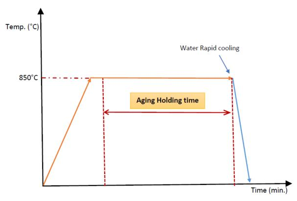
Figure II.3: scheme of applied aging treatment.
