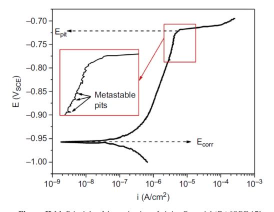
**Figure II.14:** Principle of determination of pitting Potential  $(E_p)$  [OBE 17].
