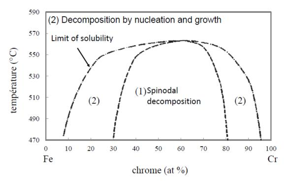
**Figure I.15:** Fe–Cr binary phase diagram [MAE 14].
