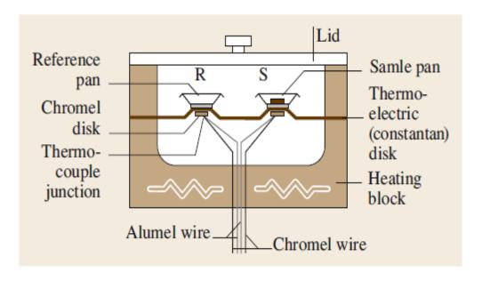
**Figure II.11 :**Schematic illustration of heat-flux DSC cell. R and S refer to reference and sample pans [KAS 17].
