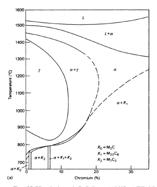
**Figure I.7:** Effect of carbon on the Fe–Cr diagram: (a) 0.05C wt% [BHA 06].
