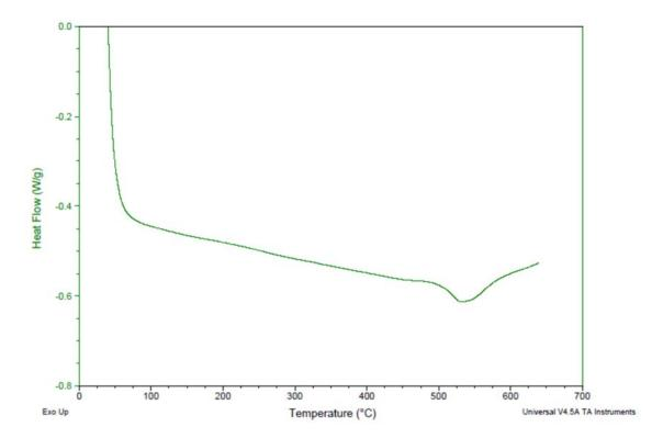
**Figure III.13:** DSC curve of heating measurement duplex stainless steel. Heating rate 30°C/min.
