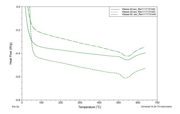
**Figure III.15:** DSC curves of heating measurement duplex stainless steel. Heating rate 30, 40 and 60°C/min.
