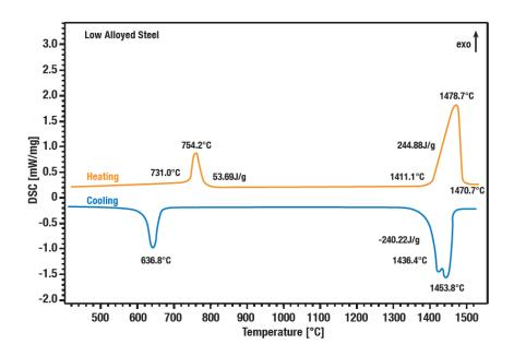
Figure II.12: Typical DSC signal for a Low Alloy Steel [LIN 20].
