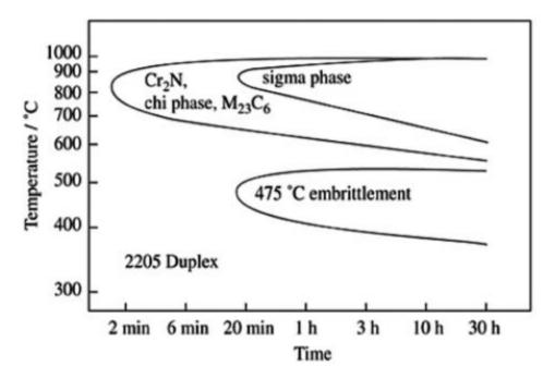
**Figure I.9:** Intermetallic phase precipitations for UNS S31803 DSS [PRA 15].
