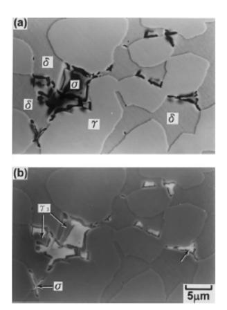
**Figure A.4:** Scanning electron micrographs showing  $\sigma$  phase located at the  $\delta/\gamma$  interface, (a) SE and (b) BS images (electrolytically etched in 10 NNaOH solution) [CHE 01].
