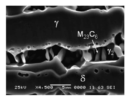
**Figure A.6:** SEM micrograph of HAZ solution treated at 1150 °C for 1 h then aged at 850 °C for 3 h [BAD 08].
