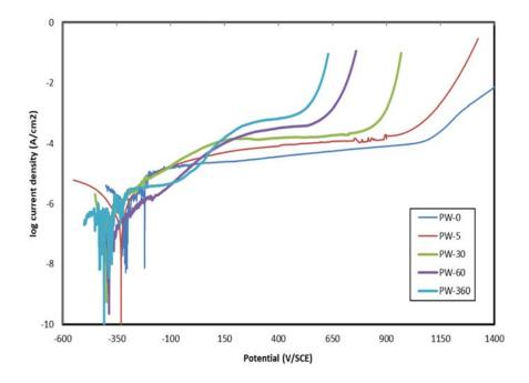
**Figure III.21:** Potentiodynamic polarization curves for the aged samples at 850°C in for different times in Produced Water solution.
