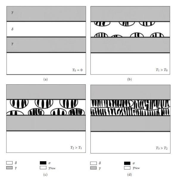
**Figure I.13:** Precipitation mechanism of the  $\sigma$  phase in UNS S31803 stainless steel [CHI 12].
