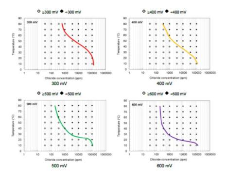
**Figure III.23:** Potential diagram for Lean Duplex SS (LDX 2101) at the different selected potentials [MAM 14].
