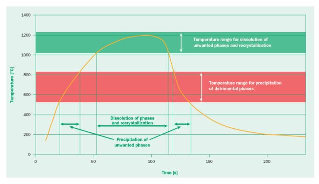
**Figure III.17:** Example of a solution annealing cycle. The critical temperature ranges are strongly dependent on the steel grade [OUT 13].
