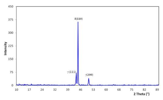
**Figure III. 2:** X-Ray diffraction pattern of the studied material in the as received condition.
