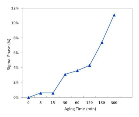
**Figure III. 7:** Variation of the volume fraction of sigma phase in UNS S31803 as a function of aging time at 850 °C.
