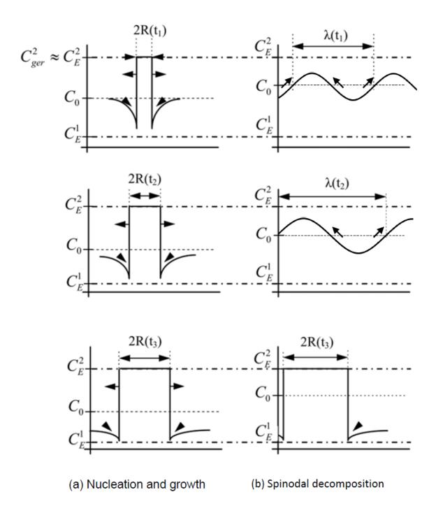
**Figure 1.16**: Formation of precipitates by a classical mechanism of nucleation and growth or by spinodal decomposition.  $C_0$ ,  $C_E^1$  and  $C_E^2$  are respectively the initial composition of phase 1 and the equilibrium compositions of phase 1 and phase 2. R is the radius of the nuclei then of the precipitates and  $\lambda$  is the wavelength of the fluctuations [MAE 14].
