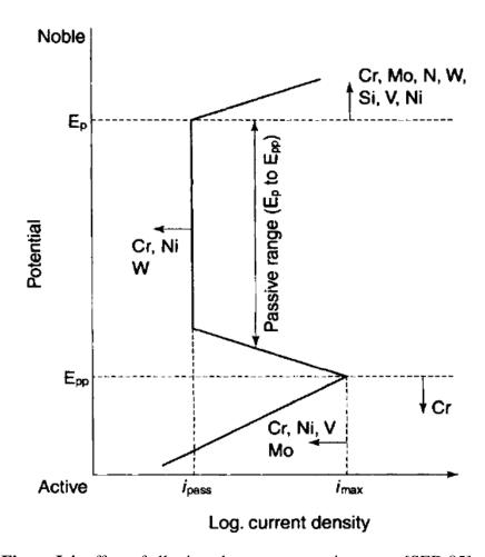
**Figure I.4:** effect of alloying elements on passive range [SED 85].
