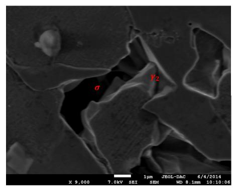
**Figure III.5:** SEM micrograph corresponding to the aged specimen at 850 °C for 360 min, Morphology of secondary austenite ( $\gamma$ 2) and sigma phase.
