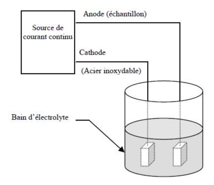
Figure II.4: Schematic for electrolytic etching cell.
