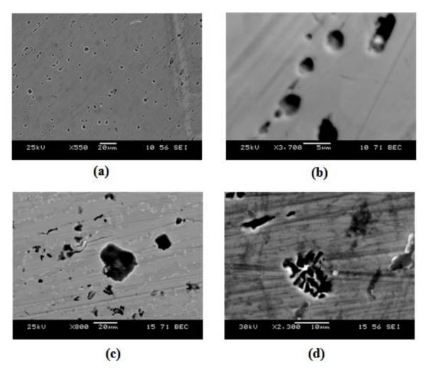
**Figure III.24:** SEM images of pitted samples (a) and (b) solution treated sample, (c) and (d) aged samples for 60 min at 850°C.
