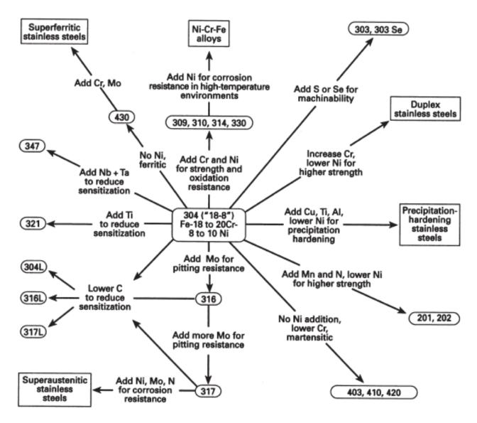
**Figure I.1:** Composition and property linkages in the stainless steel family of alloys [ASM 00].
