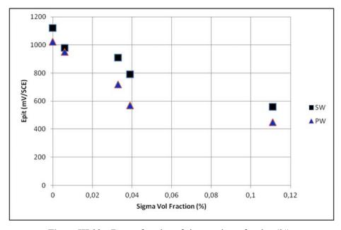
**Figure III.22**:  $E_p$  as a function of sigma volume fraction (%).
