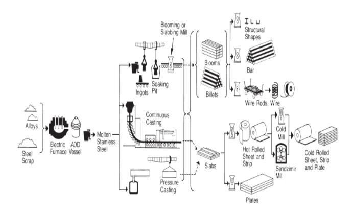
**Figure I.2:** Stainless steel manufacturing routes [ASM 00].
