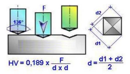
Figure II.5: Vickers Microhardness test principle.
