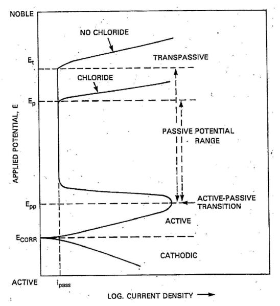
**Figure I.20:** Schematic polarization curve for a stainless steel in a sulphuric acid solution [SAI 07].
