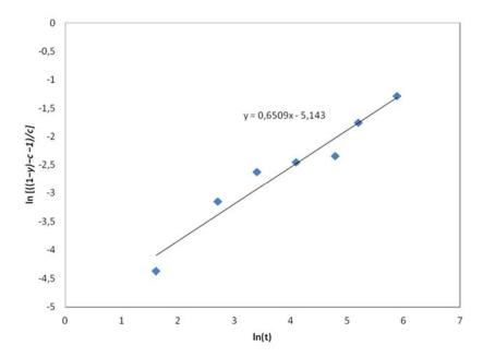
**Figure III. 10:** Application of the modified JMA model to the sigma phase precipitation during aging at 850 °C.
