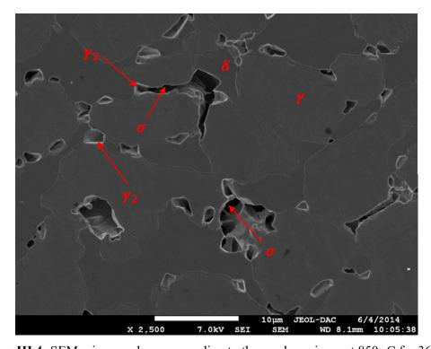
**Figure III.4:** SEM micrograph corresponding to the aged specimen at 850 °C for 360 min.
