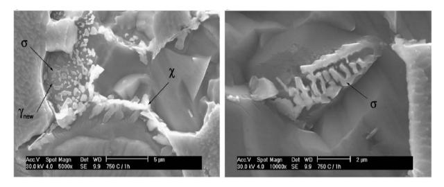
**Figure A.5:** SEM micrographs of the DSS after aging at 750 °C for 1 h. Etching: V2A-Beize [ESC 09].
