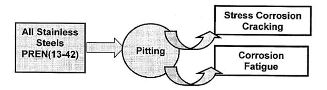
**Figure I.18:** Schematic diagram of the role of pitting [SAI 07].
