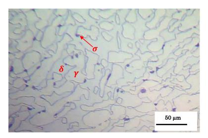
Figure III.3: Optical microstructure corresponding to the aged specimen at 850°C for 5 min.
