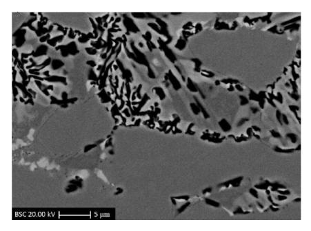
**Figure A.7:** Typical pitting morphologies of UNS S31803 DSS after polarization at 0.6M NaCl solution, aged for 6h@750°C [SAN 14].
