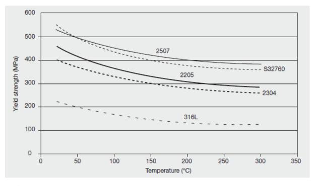
**Figure I.3:** Comparison of typical yield strength of duplex stainless steels and Type 316L between room temperature and 300°C (572°F) [IMO 09]
