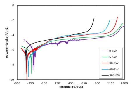
**Figure III.20:** Potentiodynamic polarization curves for the aged samples at 850°C in for different times in simulated seawater solution.
