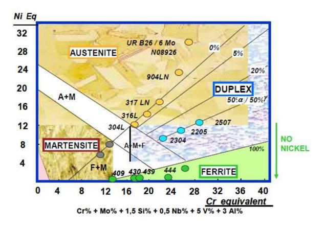
**Figure I.8:** Schaeffler diagram illustrating the Stainless Steels families positions [CHA 10]
