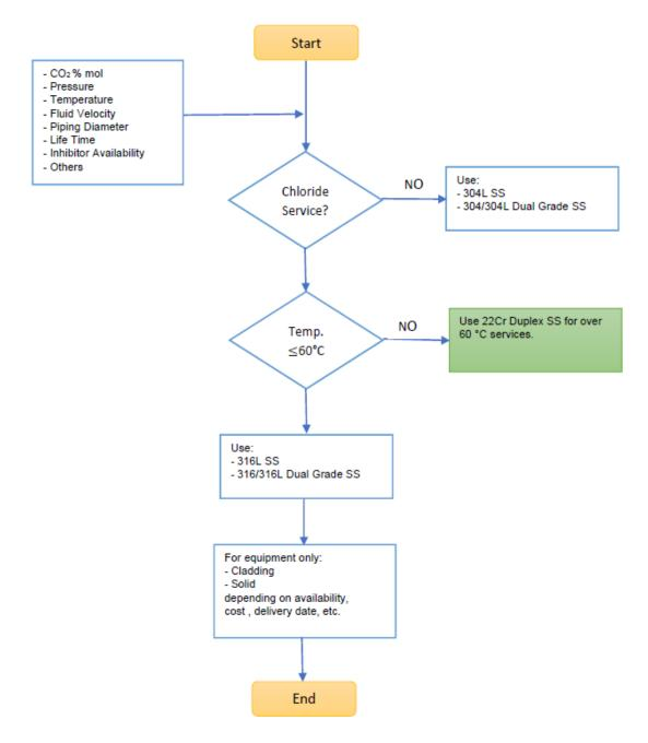
Figure II.1: Flow Diagram for Stainless Steel Materials Selection for Process Piping.
