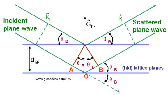
Figure II.7: Schematic illustration of Bragg condition and Bragg's law [GLO 20].
