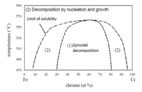
**Figure III.14:** Fe–Cr binary phase diagram [MAE 14].
