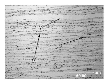
**Figure A.2:** Optical micrograph corresponding to a longitudinal section of aged DSS at 850°C for 2h, electrolytically etched in 30% KOH solutions [DEN09].
