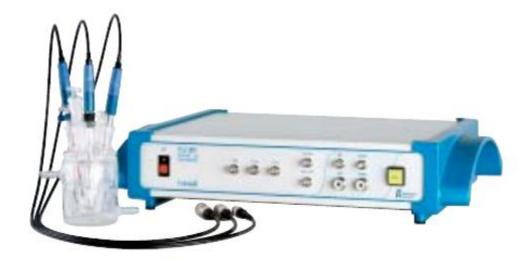
**Figure II. 16:** The VOLTALAB PGZ-301 potentiostat.
