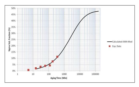
**Figure III. 11:** Comparison between experimental data and the modified JMA analysis of sigma volume fraction during aging at 850°C.
