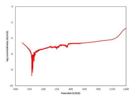
**Figure III. 18:** Potentiodynamic polarization curves for the solution treated sample in simulated seawater solution.
