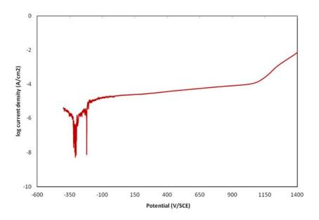
**Figure III. 19:** Potentiodynamic polarization curves for the solution treated sample in Produced water solution.
