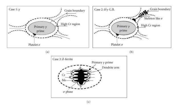
**Figure I.12:** Schematic diagram of the  $\sigma$  phase precipitation [CHI 12].
